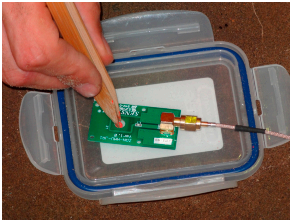
Figure 3. An artificial gravel particle used in the first experiment shown within the Radio-Frequency Identification reader.
