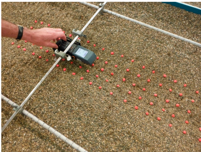
Figure 5. The locations of the array of 100 particles being read by the RFID reader before the second experiment.
