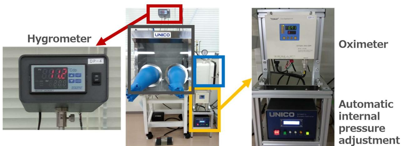
Figure 3.1 The glove box system used for sample preparation.
