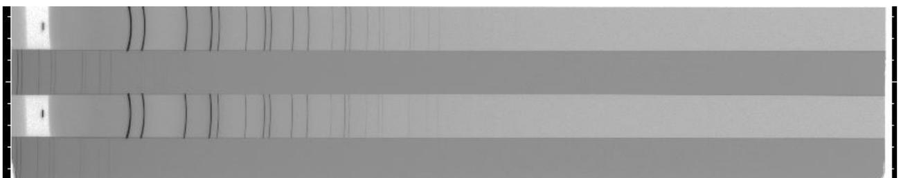
(d) 2-dimensional diffraction data of aluminum at 500 and 600 K.
