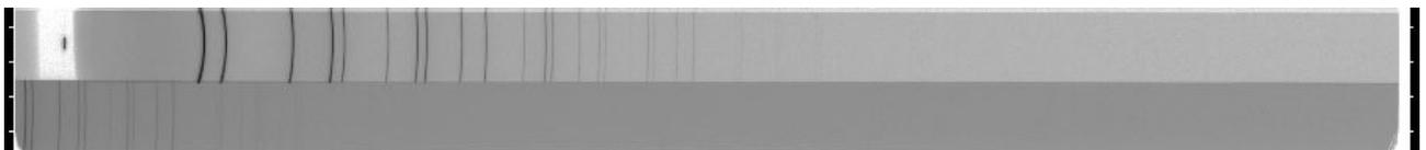
(c) 2-dimensional diffraction data of aluminum at 400 K.
