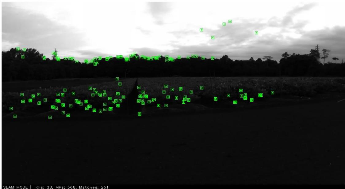
Figure 5.13. ORB features detected by ORB-SLAM system using ZED camera to navigate the EPV
