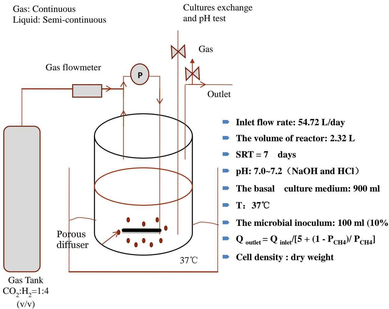
Fig. 2-1 Schematic diagram of the semi-continuous methane fermentation system.
