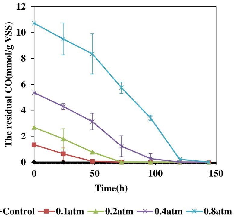
Fig. 3-8 Effect of CO partial pressures (atm) on CO consumption by AGS.
