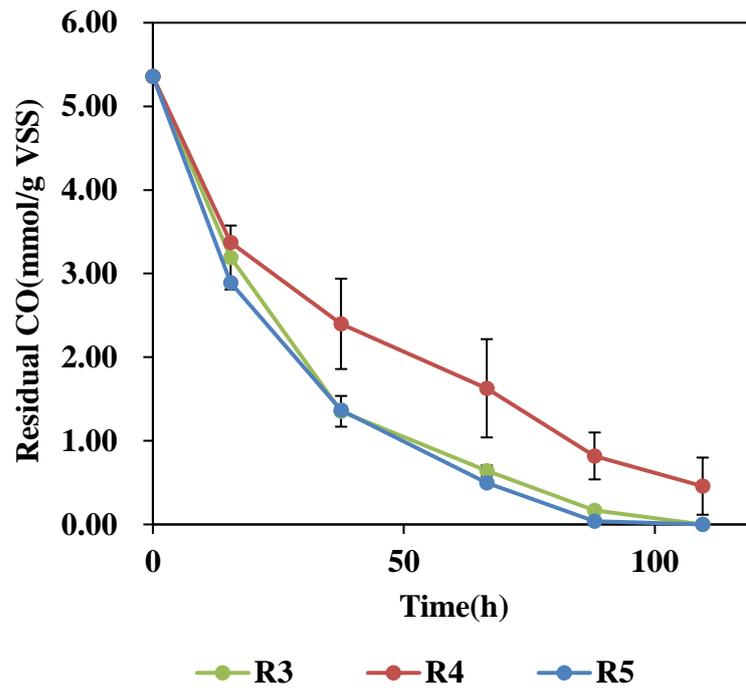
Fig. 3-4 Anaerobic biomethanation potential of AGS at 37°C: CO consumption (R3-CO/N<sub>2</sub>, R4-CO/H<sub>2</sub>; R5-CO/CO<sub>2</sub>/H<sub>2</sub>)
