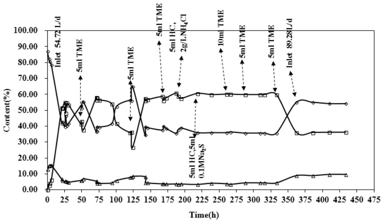
Fig. 2-5 Changes in outlet CH<sub>4</sub> content from the semi continuous reactor. H<sub>2</sub> (◇), CH<sub>4</sub> (□), CO<sub>2</sub>
