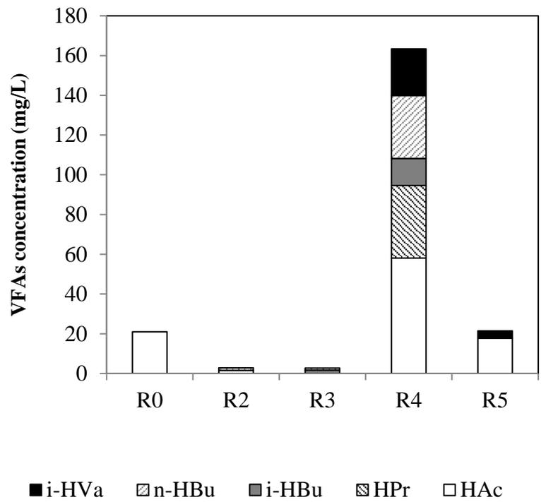
Fig. 3-6 Anaerobic biomethanation potential of AGS at 37°C: VFAs production (R0-control, R1-sodium acetate, R2-H<sub>2</sub>/CO<sub>2</sub>, R3-CO/N<sub>2</sub>, R4-CO/H<sub>2</sub>; R5-CO/CO<sub>2</sub>/H<sub>2</sub>)
