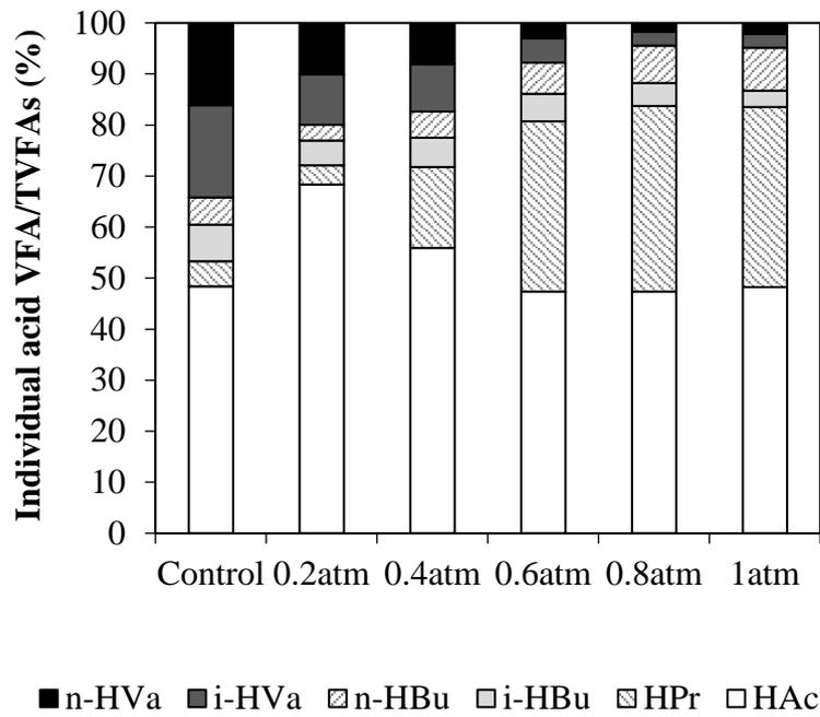
Fig. 3-10 Effect of CO partial pressures (atm) on percentage of individual VFA species to the total VFAs (TVFAs) in the presence of BES at 37°C on day 7.
