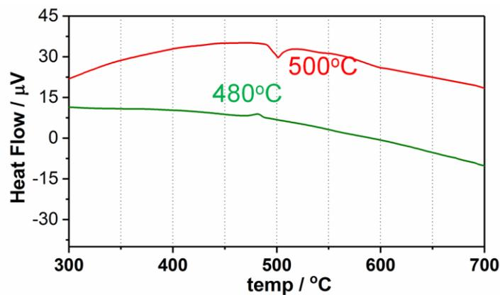
Fig. 4-4 DTA profile of  $\text{Nd}_{80}\text{Ga}_{15}\text{Cu}_5$  alloy; heating curve is displayed in red and cooling curve in green.
