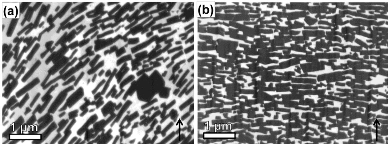
Fig. 6-14 BSE-SEM images of surface (a) and center (b) regions of the Nd-Ga-Cu diffusion-processed magnets under expansion constraint with  $t=0$  mm. The observation direction was along the easy axis as indicated by the arrows.
