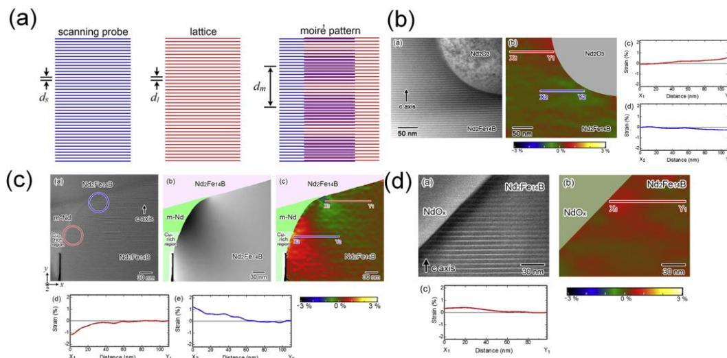
Fig. 1-8 Strain measurement using artificial moiré fringes. (a) Schematic representation of the construction of artificial moiré fringes; Strain measurement from (b)  $\text{Nd}_2\text{O}_3/\text{Nd}_2\text{Fe}_{14}\text{B}$ , (c) metallic-Nd/ $\text{Nd}_2\text{Fe}_{14}\text{B}$  (including a Cu-rich Nd-rich GB/ $\text{Nd}_2\text{Fe}_{14}\text{B}$ ), (d)  $\text{NdO}_x/\text{Nd}_2\text{Fe}_{14}\text{B}$  interfaces [31].
