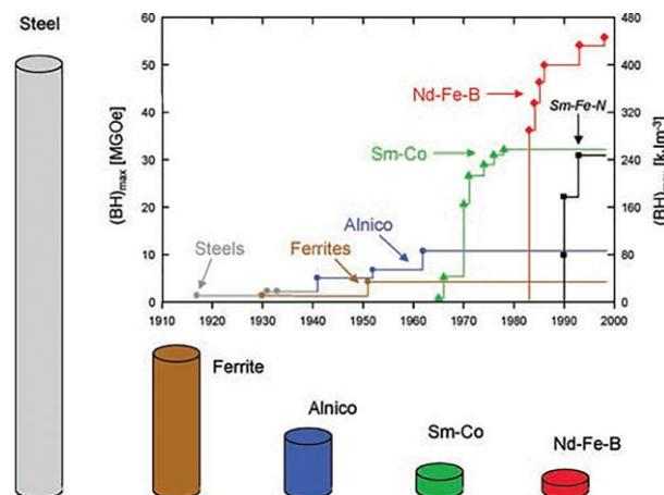
Fig. 1-1 Development in the energy density  $(BH)_{\max}$  at room temperature of hard magnetic materials in the 20<sup>th</sup> century and presentation of different types of materials with comparable energy product [1].
