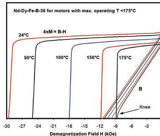
Fig. 1-2 Demagnetization curves in the 2<sup>nd</sup> quadrant at various temperatures of Nd-Dy-Fe-B used for motors
