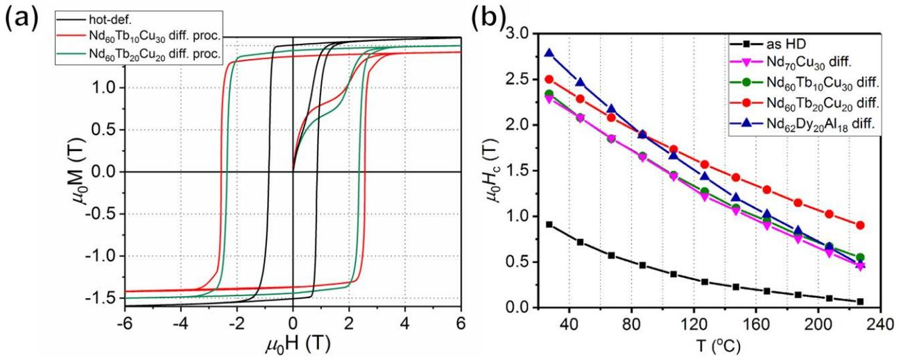
Fig. 5-7 (a) Hysteresis loops of the hot-deformed,  $\text{Nd}_{60}\text{Tb}_{10}\text{Cu}_{30}$ , and  $\text{Nd}_{60}\text{Tb}_{20}\text{Cu}_{20}$  diffusion-processed magnets; (b) temperature dependence of coercivity of the hot-deformed,  $\text{Nd}_{60}\text{Tb}_{10}\text{Cu}_{30}$ , and  $\text{Nd}_{60}\text{Tb}_{20}\text{Cu}_{20}$  diffusion-processed magnets, in comparison with Nd-Cu (Chapter 3) and Nd-Dy-Al (Chapter 5.3.1) diffusion-processed magnets.
