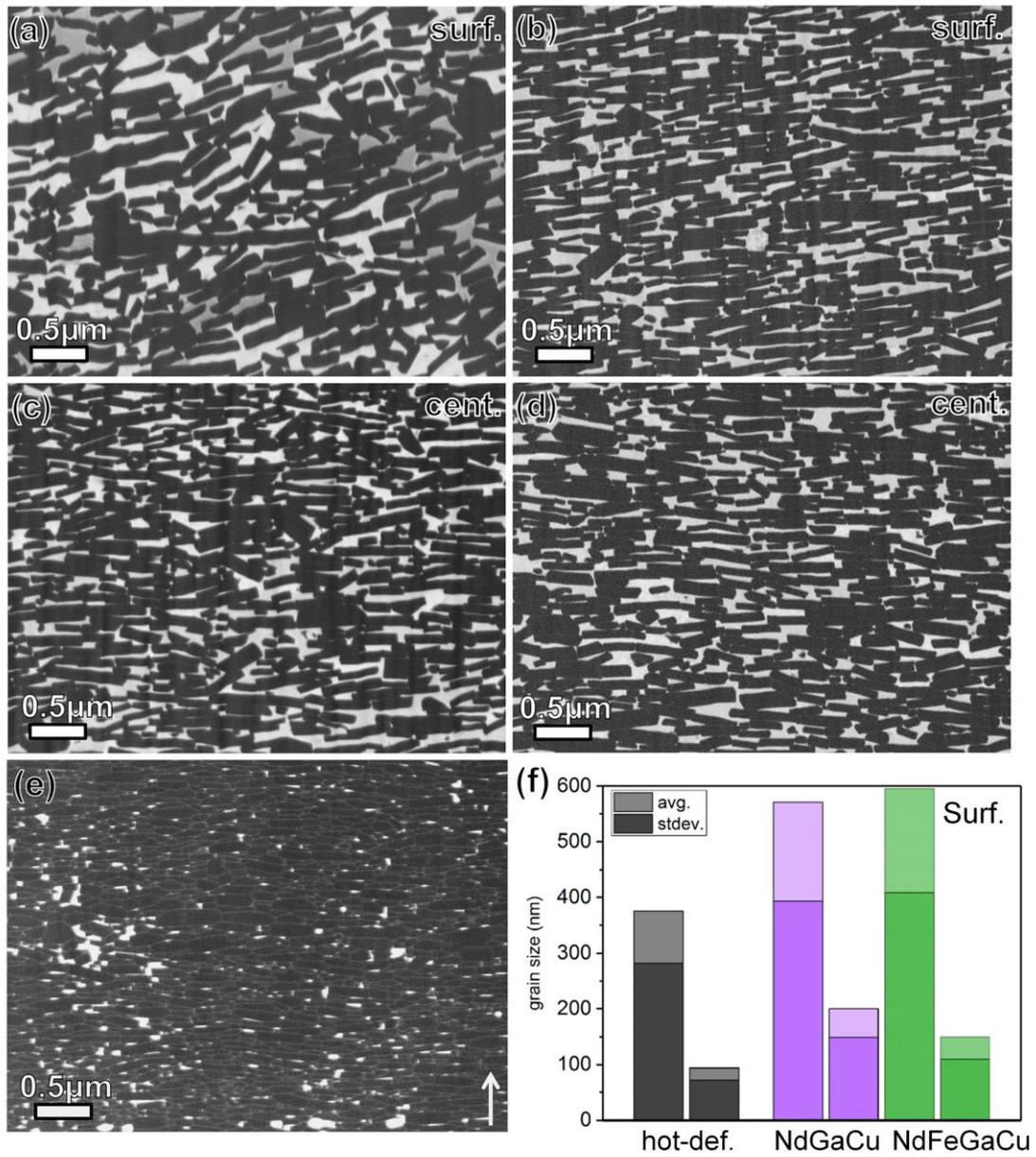
Fig. 4-8 BSE SEM images of (a) surface and (c) center regions of  $\text{Nd}_{80}\text{Ga}_{15}\text{Cu}_5$  diffusion-processed, (b) surface and (d) center regions of  $\text{Nd}_{62}\text{Fe}_{14}\text{Ga}_{20}\text{Cu}_4$  diffusion-processed magnets. (e) hot-deformed magnets; (f) Grain size statistics of surface regions of the hot-deformed, Nd-Ga-Cu and Nd-Fe-Ga-Cu diffusion-processed magnets.
