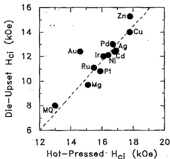
Fig. 1-10 Coercivity ( $H_{ci}$ ) for die-upset versus hot-pressed magnets containing the same additive. The additive-free magnet is denoted by MQ. The broken line is a guide to the eye, indicating the general relationship between the coercivity of a die-upset magnet and its hot precursor [64].
