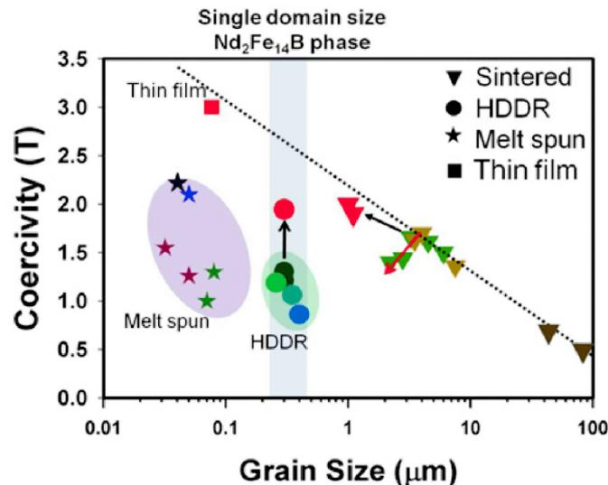
Fig. 1-11 Empirical plot of coercivity in the relationship with the mean grain size of NdFeB magnets [77].
