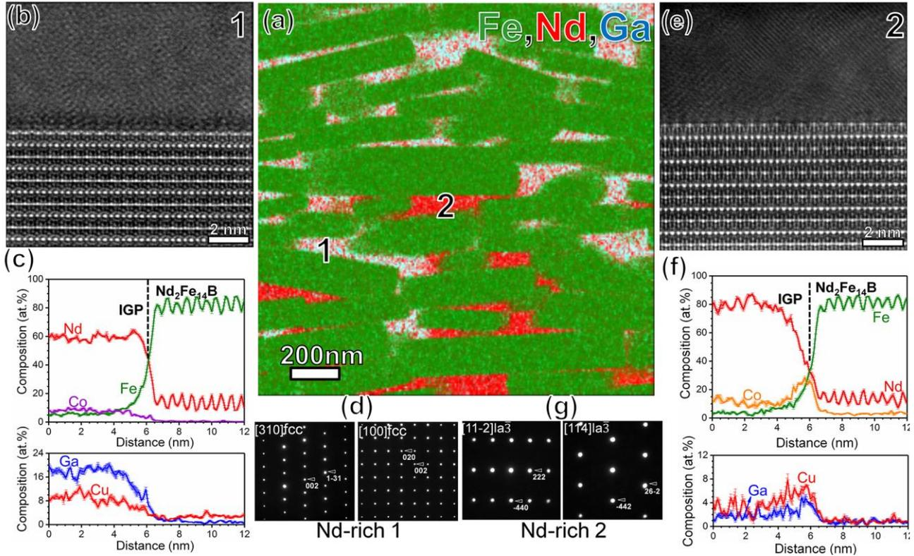
Fig. 4-10 (a) Superimposed EDS elemental map of Fe, Nd and Ga, (b) Nd-rich phase 1/ Nd<sub>2</sub>Fe<sub>14</sub>B interface, (c) line-scan profile across the interface shown in b, (d) NBED of Nd-rich phase 1, (e) Nd-rich phase 2/ Nd<sub>2</sub>Fe<sub>14</sub>B interface, (f) line-scan profile across the interface shown in e, (g) NBED of Nd-rich phase 2 from Nd<sub>80</sub>Ga<sub>15</sub>Cu<sub>5</sub> diffusion-processed sample.
