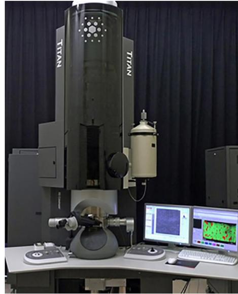
Fig. 2-4 Cs-corrector equipped FEI Titan G2 80-200.
