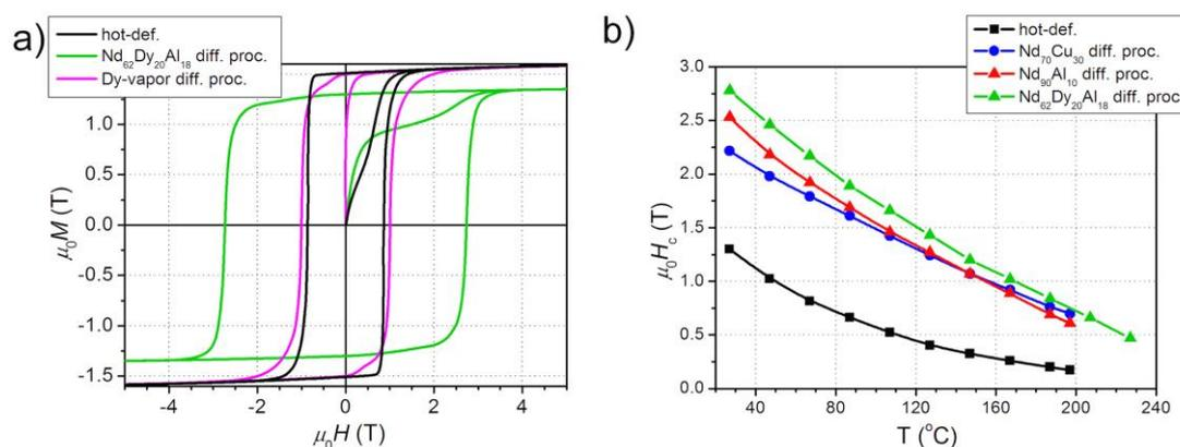
Fig. 5-1 (a) Hysteresis loops of the hot-deformed,  $\text{Nd}_{62}\text{Dy}_{20}\text{Al}_{18}$  and Dy-vapor diffusion-processed samples; (b) Temperature dependence of coercivity of the hot-deformed,  $\text{Nd}_{70}\text{Cu}_{30}$ ,  $\text{Nd}_{90}\text{Al}_{10}$  and  $\text{Nd}_{62}\text{Dy}_{20}\text{Al}_{18}$  diffusion-processed samples.
