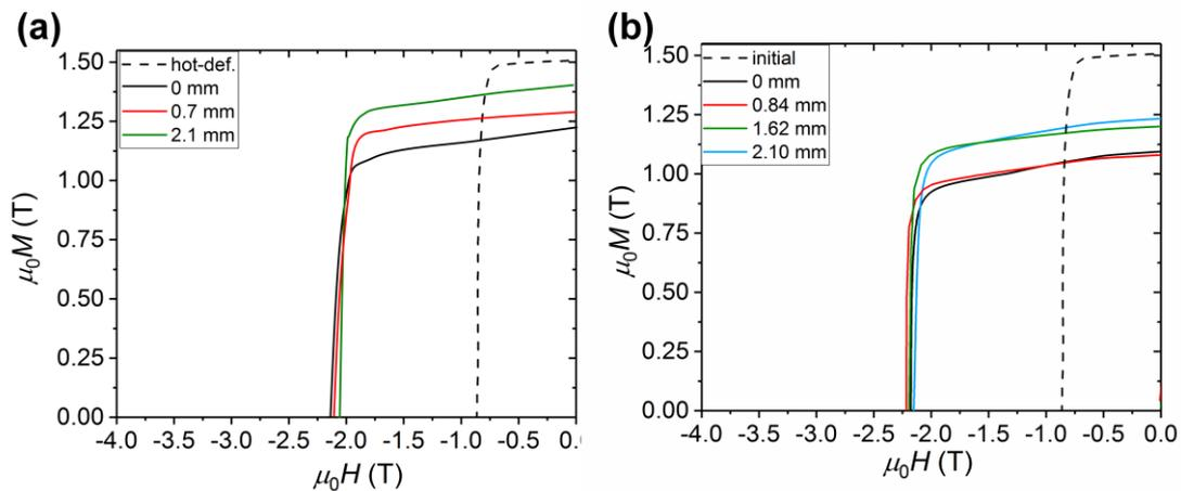
Fig. 6-11 Demagnetization curves of the Nd-Ga-Cu diffusion-processed magnets under expansion constraint with  $t=0.1\text{mm}$  (a) and without expansion constraint applied (b) measured for the specimen taken from different distances from surfaces of the magnets.
