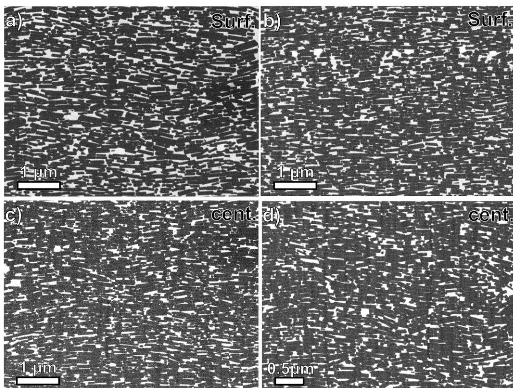
Fig. 5-8 BSE-SEM images of surface and center regions of  $\text{Nd}_{60}\text{Tb}_{10}\text{Cu}_{30}$  (a, c), and  $\text{Nd}_{60}\text{Tb}_{20}\text{Cu}_{20}$  (b, d) diffusion-processed magnets.
