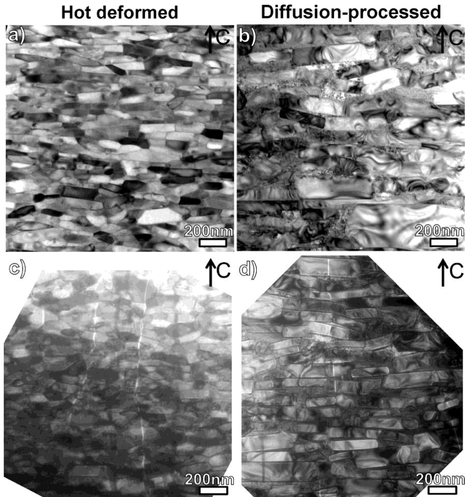
Fig. 3-4 BF-TEM images and Lorentz TEM images of the hot-deformed (a,c) and the  $\text{Nd}_{90}\text{Al}_{10}$  diffusion-processed (b,d) samples. The observation direction is along the easy-axis lying in-plane.
