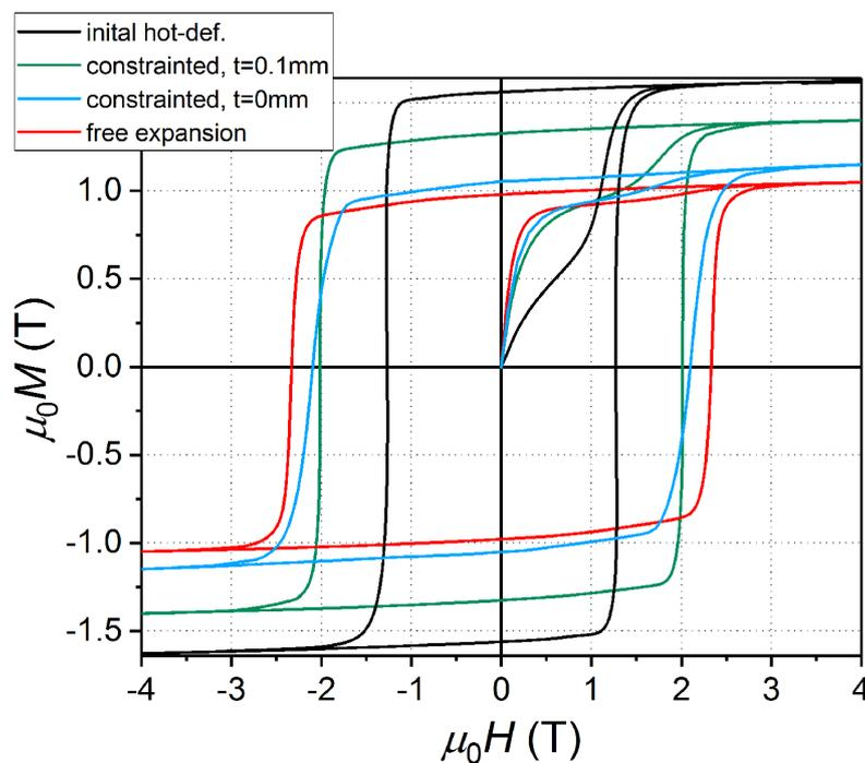
Fig. 6-10 Hysteresis loops of the initial hot-deformed and Nd-Ga-Cu diffusion-processed magnets.
