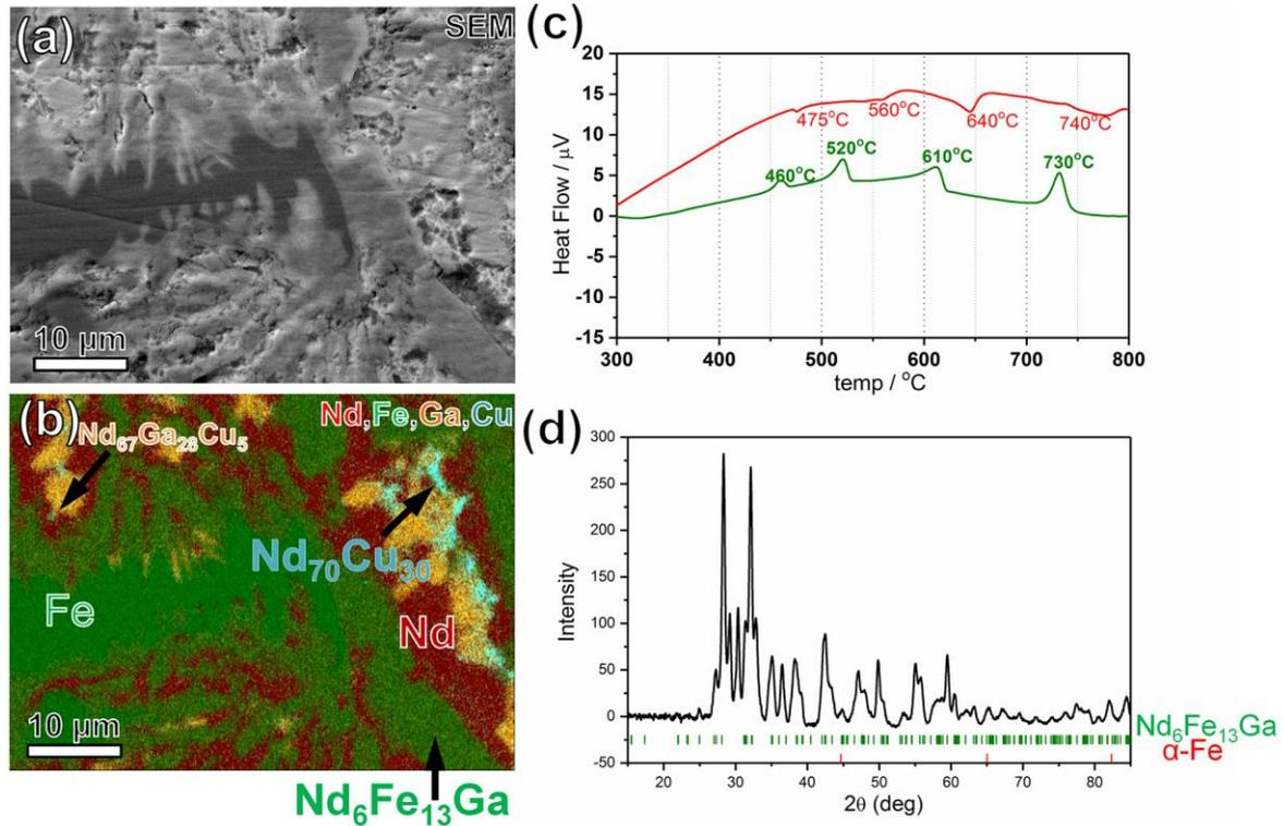
Fig. 4-3 (a) BSE-SEM image and (b) the superimposed EDS elemental maps of Nd, Fe, Ga and Cu from the same region in  $\text{Nd}_{62}\text{Fe}_{14}\text{Ga}_{20}\text{Cu}_5$  ingot; (c) DTA heating (in red) and cooling (in green) curves and (d) XRD  $2\theta$  scan profile of  $\text{Nd}_{62}\text{Fe}_{14}\text{Ga}_{20}\text{Cu}_5$  ingot.
