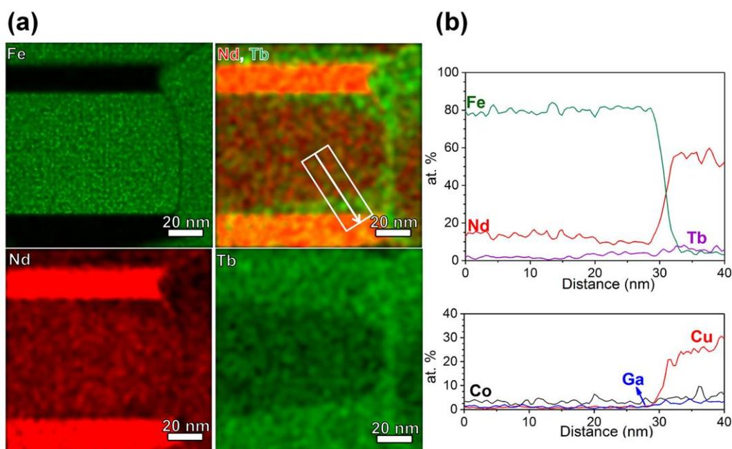
Fig. 5-12 BF-TEM, HAADF-STEM images of  $\text{Nd}_{60}\text{Tb}_{20}\text{Cu}_{20}$  diffusion-processed sample and EDS elemental maps of Nd- $L_{\alpha}$ , Fe- $K_{\alpha}$ , Ga- $K_{\alpha}$ , Tb- $M_{\alpha}$ , Cu- $K_{\alpha}$ , Co- $K_{\alpha}$  taken from the very same region in the HAADF image.
