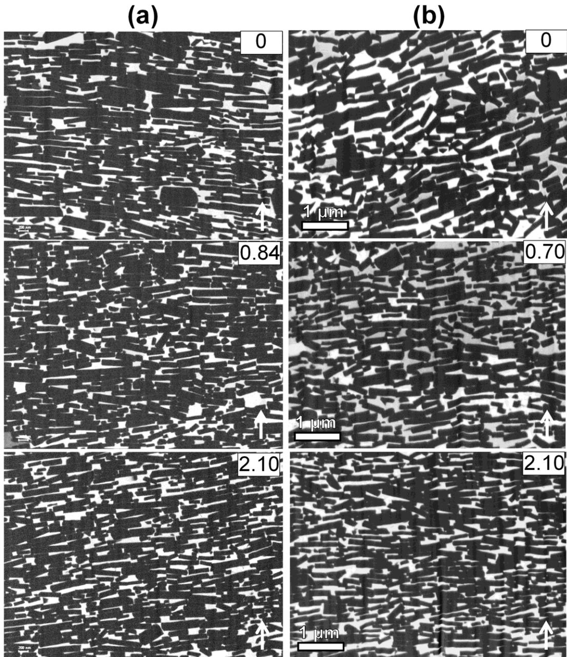
Fig. 6-12 BSE-SEM images of the Nd-Ga-Cu diffusion-processed magnets under expansion constraint with  $t=0.1\text{mm}$  (a) and without expansion constraint applied (b) taken from regions within the same distances from surfaces of the magnets as the vsm specimens. The observation direction is along c-axis in-plane; as indicated by the arrows.
