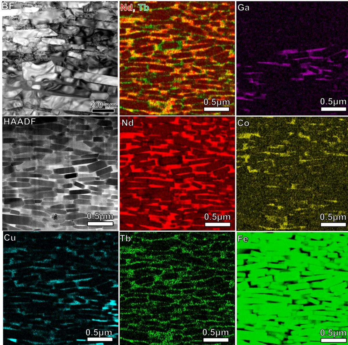
Fig. 5-11 BF-TEM, HAADF-STEM images of  $\text{Nd}_{60}\text{Tb}_{20}\text{Cu}_{20}$  diffusion-processed sample and EDS elemental maps of  $\text{Nd-L}_{\alpha}$ ,  $\text{Fe-K}_{\alpha}$ ,  $\text{Ga-K}_{\alpha}$ ,  $\text{Tb-M}_{\alpha}$ ,  $\text{Cu-K}_{\alpha}$ ,  $\text{Co-K}_{\alpha}$  taken from the very same region in the HAADF image.
