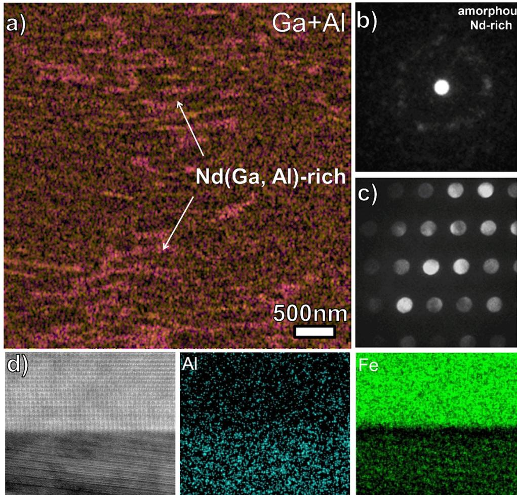
Fig. 3-7 (a) STEM-EDS elemental mapping images of Ga overlapped with Al maps of NdAl-infiltrated sample. The selected analysis peaks for the elemental maps are Fe  $K\alpha$ , and Co  $K\alpha$ . (b,c) NBED patterns taken from amorphous and Nd(Fe,Al)<sub>2</sub> intergranular Nd-rich regions, respectively; (d) STEM-HAADF image and EDS maps taken from the Nd(Fe,Al)<sub>2</sub> phase.
