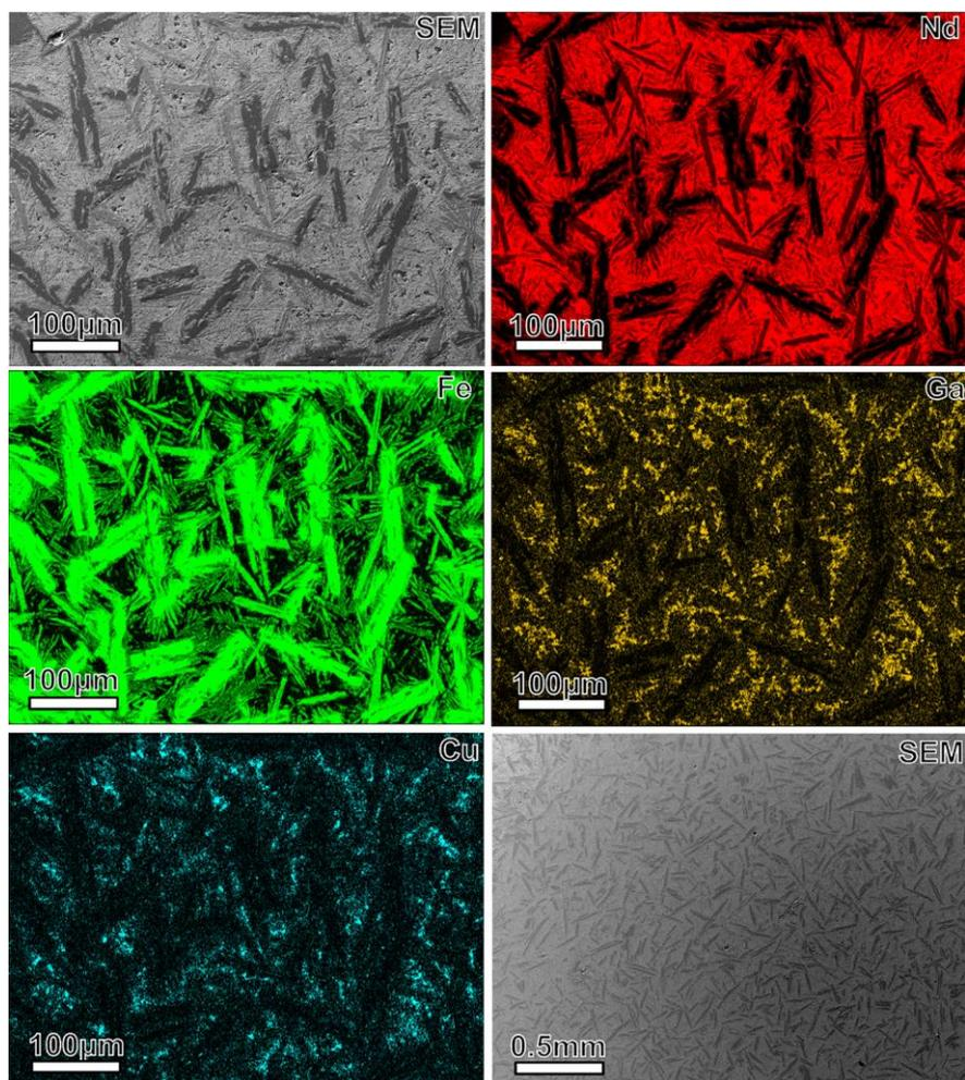
Fig. 4-2 BSE-SEM image and EDS elemental maps of Nd, Fe, Ga and Cu from the same region in the as-cast  $\text{Nd}_{62}\text{Fe}_{14}\text{Ga}_{20}\text{Cu}_4$  ingot prepared by induction-melting with steel plate-mould.
