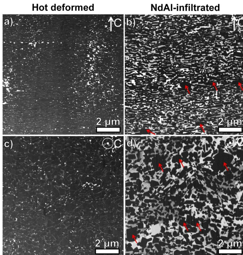
Fig. 3-3 BSE-SEM images of the hot-deformed (a,c) and the  $\text{Nd}_{90}\text{Al}_{10}$  diffusion-processed (b,d) samples. The observation direction is along the easy-axis lying in-plane (a,b) and out-of-plane in (c,d).
