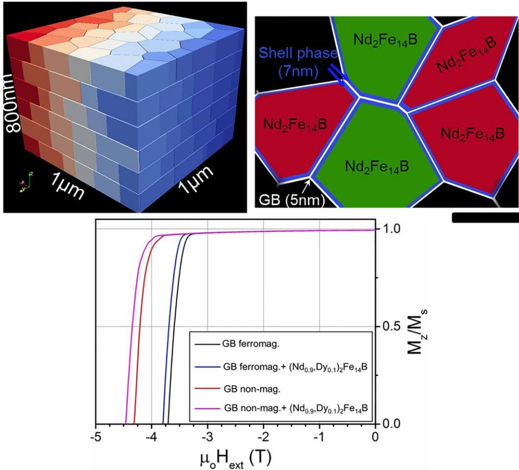
Fig. 6-8 (a) The microstructure of a finite element model with a size of  $1 \times 1 \times 0.8 \mu\text{m}^3$ , showing the grain size. (b) The schematic image of the microstructure of the modeled hot-deformed magnet. (c) The demagnetization curves of the simulated samples with different magnetization (0 and 0.5 T) and w/o Dy-rich shell phase.
