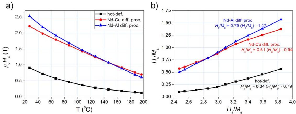
Fig. 3-2 (a) Temperature dependence of coercivity of the hot-deformed, Nd-Al and Nd-Cu diffusion-processed samples, (b) dependence of  $H_c/M_s$  on  $H_a/M_s$  of the hot-deformed, Nd-Al and Nd-Cu diffusion-processed samples. Micromagnetic parameters  $\alpha$  and  $N_{\text{eff}}$  are calculated from the slope and intercept of the linear fit of these plots, respectively.
