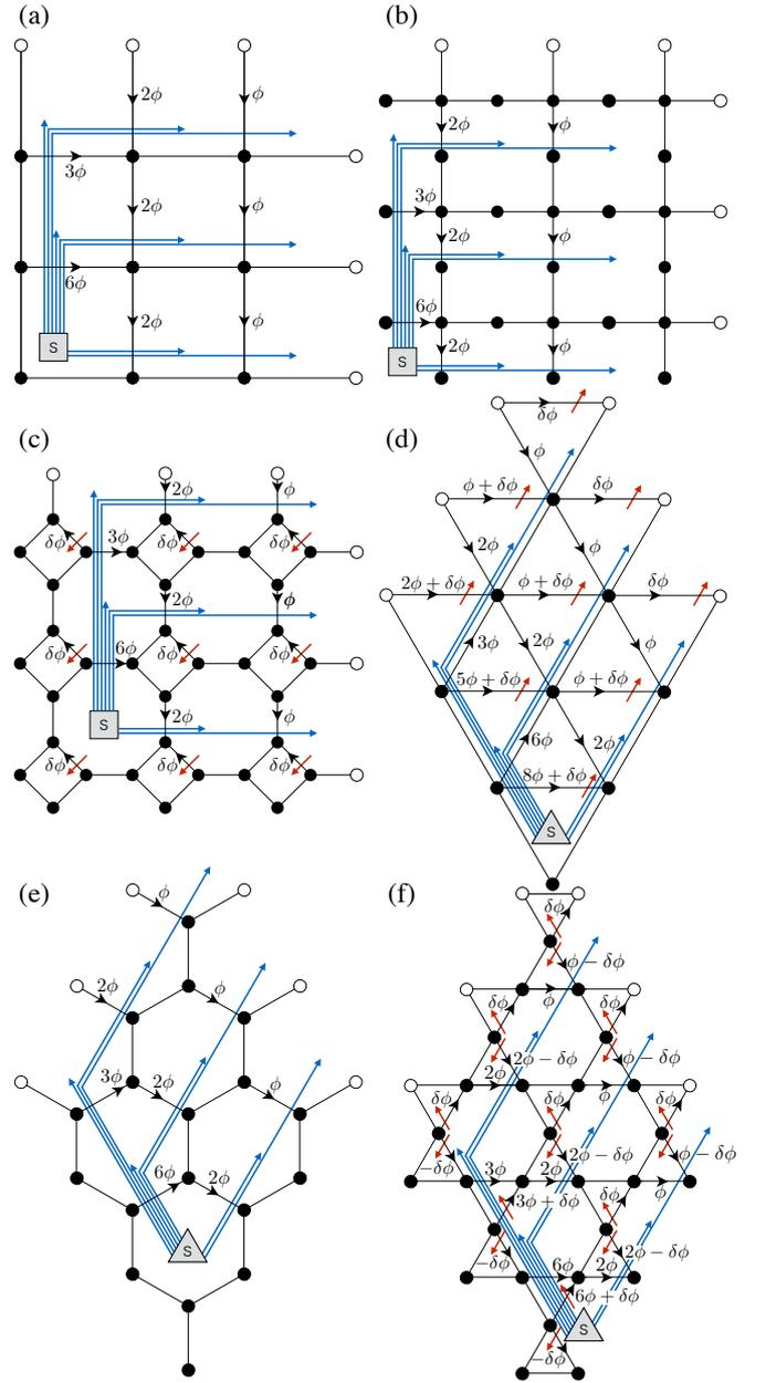
**Fig. 1.** (Color online) Sketches of  $3 \times 3$  (a) square, (b) Lieb, (c) square-octagon, (d) triangular, (e) honeycomb and (f) kagome lattices with the string gauge under periodic boundary condition.
