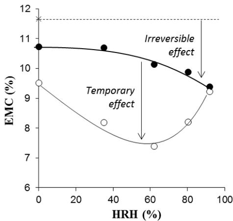
**Figure 1:** Effects of HRH on the EMC at 25°C and 60% RH of artificially aged wood.
