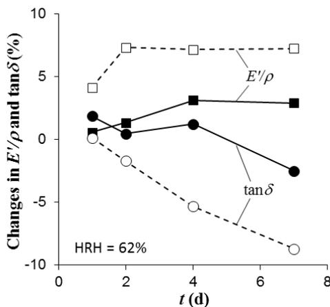
**Figure 2:** Changes in  $E'/\rho$  and  $\tan\delta$  due to artificial ageing at 120°C and 62% HRH with the elapse of heating time ( $t$ ).
