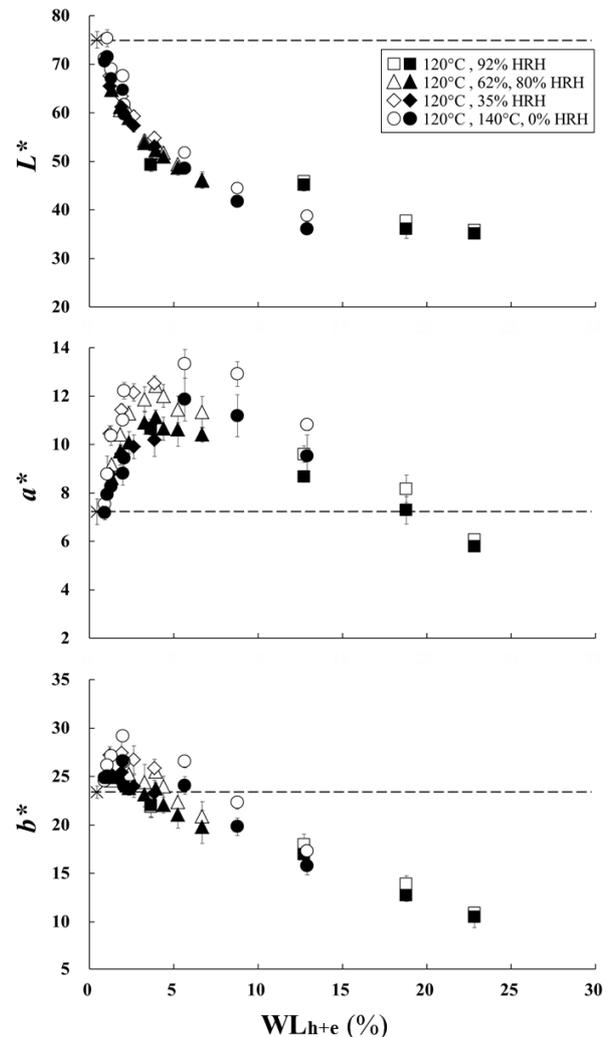
**Figure 4:** Changes in  $L^*$ ,  $a^*$  and  $b^*$  values due to artificial ageing and extraction in water plotted against  $WL_{h+e}$ . Crosses and dashed lines, the values of unmodified wood; error bars, standard deviations; open symbols, artificially aged; closed symbols, artificially aged and extracted in water
