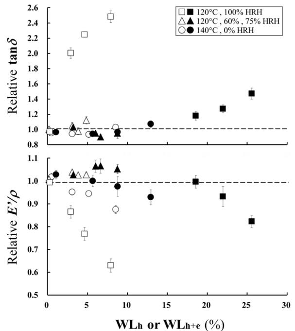
**Figure 3:** Relative  $\tan\delta$  and  $E'/\rho$  values of artificially aged wood as a function of  $WL_h$  or  $WL_{h+e}$ .
