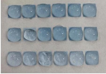
FIGURE 11: CA hydrogel on hydrophilic areas on hydrophilic/hydrophobic patterned paper.
