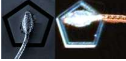
Fig. 2 (Colour online) A scanning ion microscopy image of Sample 1 with current bias feed on the middle (left) and an optical microscope image of Sample 2 with current bias feed along an edge (right).
