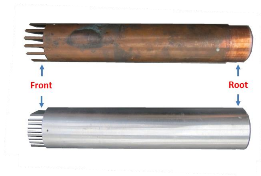
Figure 3-4 The cold head of FPSC with different materials (aluminium and copper)
