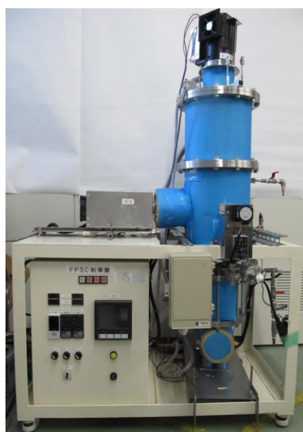
Figure 2-5 The Stirling cooler system
