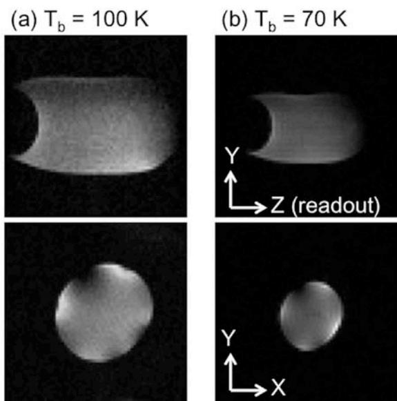
FIG. 3. MR images of  $\text{CuSO}_4$ -doped water in an NMR sample tube acquired using a 3D spin echo sequence at  $T_b$  of (a) 100, and (b) 70 K, respectively.
