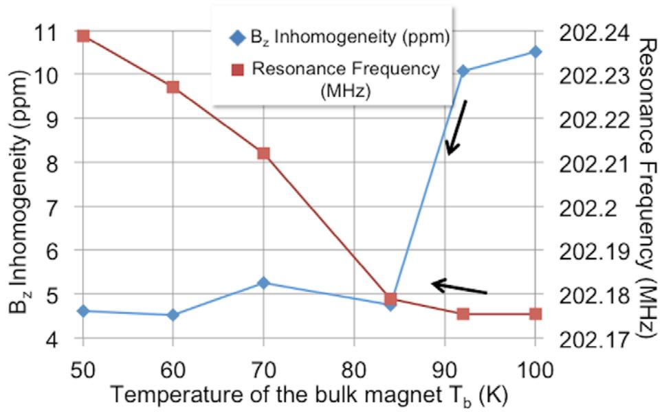
FIG. 2. Inhomogeneity of the  $B_z$  (PP) and the resonance frequency (MHz) plotted against  $T_b$  during the cooling process.
