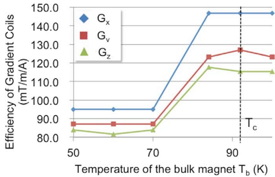
FIG. 4. Efficiencies of the gradient coils plotted against  $T_b$  during the cooling process.
