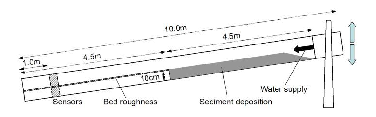
Figure 1 Experimental setup.
