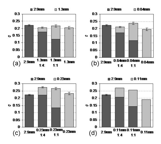
Figure 3 Sediment concentrations for the (a) 1.3-, (b) 0.84-, (c) 0.23-, and (d) 0.11-mm sediment particle experiments. Monogranular experiments and mixing ratios of 1:4 and 1:1 are shown in each column. The bars on the left in all figures indicate the sediment concentration for the uniform 2.9-mm particle experiments.
