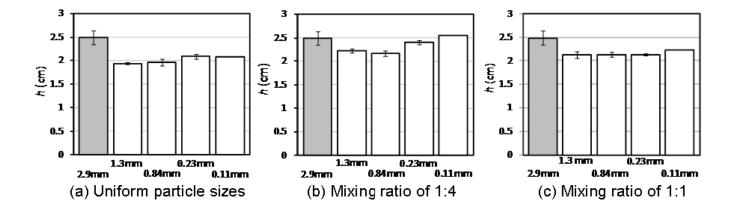
Figure 4 Flow depth for (a) uniform particle sizes and mixing ratios of (b) 1:4 and (c) 1:1. The bars to the left in (b) and (c) indicate the flow depth for the uniform 2.9-mm particle experiments as a reference.
