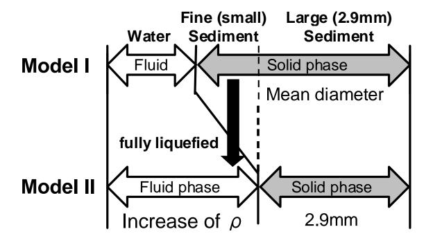
Figure 2 Schematic diagrams of Models I and II. When the fine sediment is involved (liquefied) in the pore fluid, representative sediment particle size, sediment concentration, and density of the pore fluid change.
