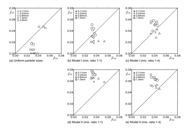
Figure 5 Relationship between the experimental and theoretical friction coefficients for (a) uniform particle sizes (Model I), mixing ratios of (b) 1:1 and (c) 1:4 with Model I, and mixing ratios of (d) 1:1 and (e) 1:4 with Model II.
