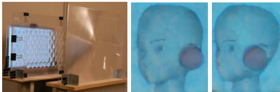
Figure 3: Prototype of coarse integral volumetric imaging (left) and the images observed from two different viewpoints with the prototype system (middle and right).
