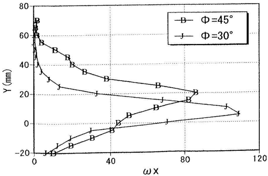
Figure 8.11 Mean vorticity in spanwise direction at  $X = 110$  mm ( $U_0 = 6.5$  m/s,  $VR = 9.5$ ,  $D_f = 2$  mm).
