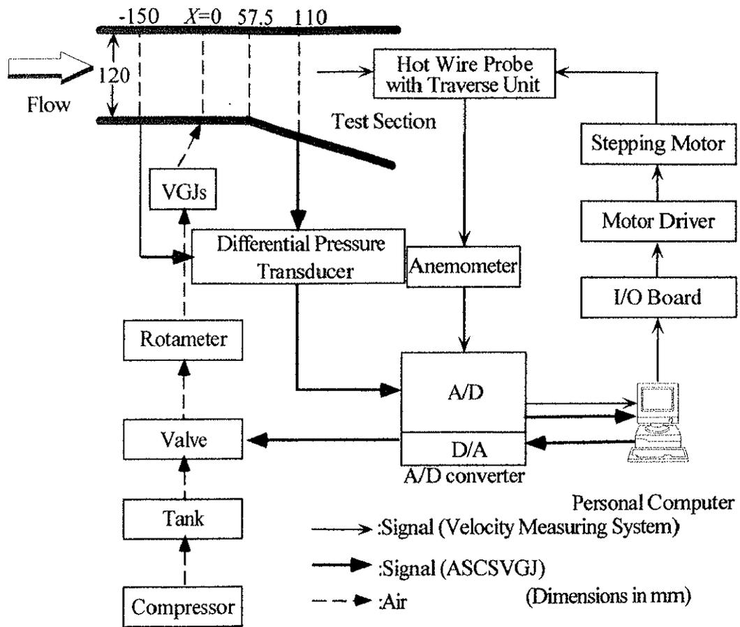
Figure 8.2 Schematic diagram of ASCSVGJ.
