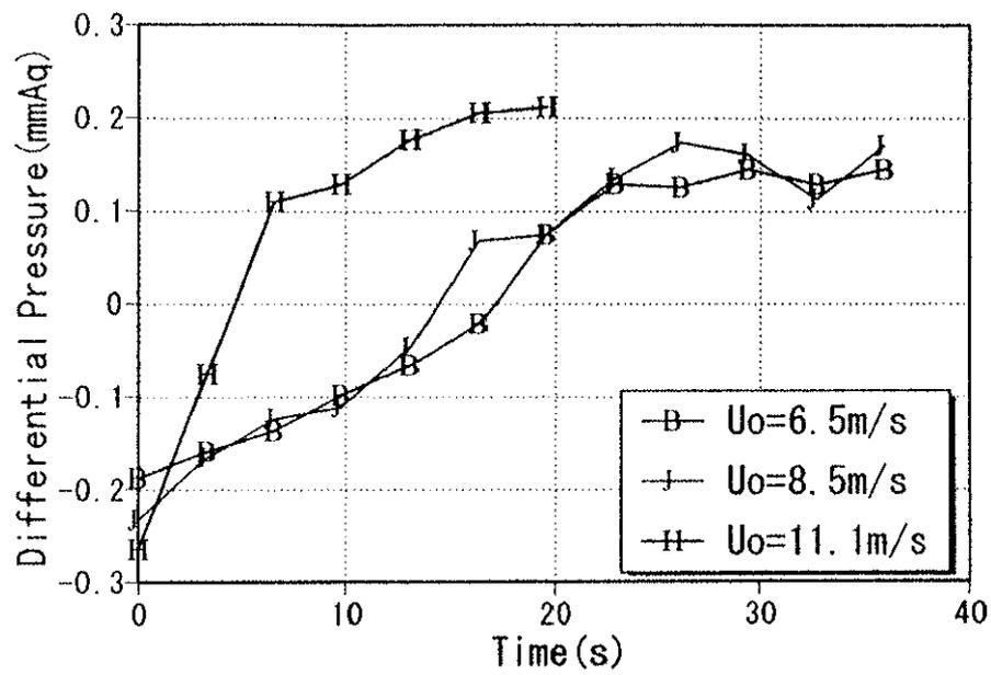
Figure 8.4 Variation of differential pressure under control.
