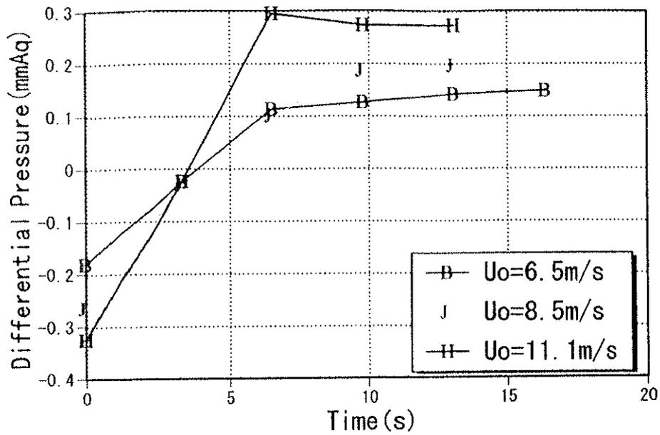
Figure 8.10 Variation of differential pressure under control ( $\phi = 30$  deg,  $D_f = 2$  mm).
