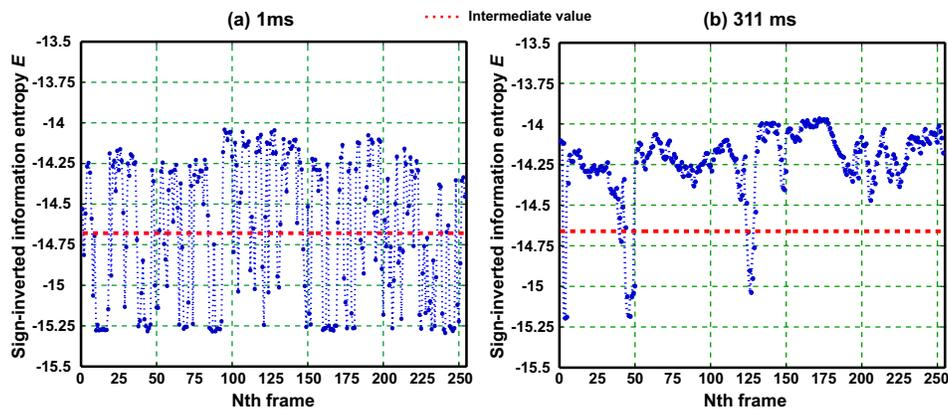
Fig. 6. Evaluation function of each frame for the integration times of (a)  $1 \text{ ms}$  and (b)  $311 \mu\text{s}$ . The result obtained for  $1 \text{ ms}$  shows a lot of missing frames due to the motion artifact in quantitative comparison to that for  $311 \mu\text{s}$ .
