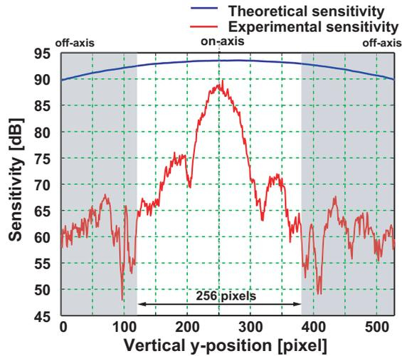
Fig. 10. Lateral position dependence of the sensitivity. Theoretical distribution of the sensitivity calculated from the Gaussian intensity profile of the line illumination on the sample (blue line). Experimental distribution of the sensitivity obtained using an achromatic lens and a mirror (red line).
