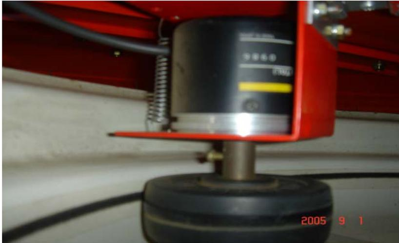
Fig. 5.5 The incremental rotary encoder used in the autonomous tractor
