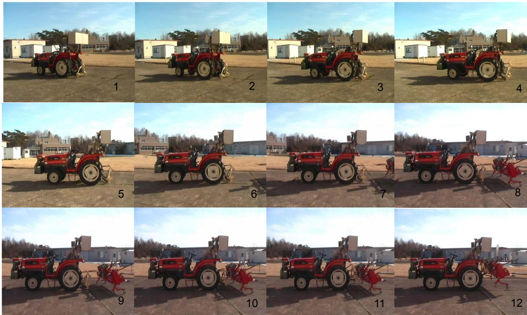
Fig. 9.7 Stages of automatic coupling with the implement using single reflector (Implement at left)
