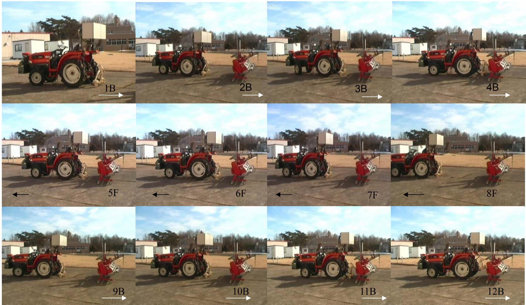
Fig. 9.10 Stages of automatic coupling in the sequential traveling with the implement using two reflectors (Implement at right)
