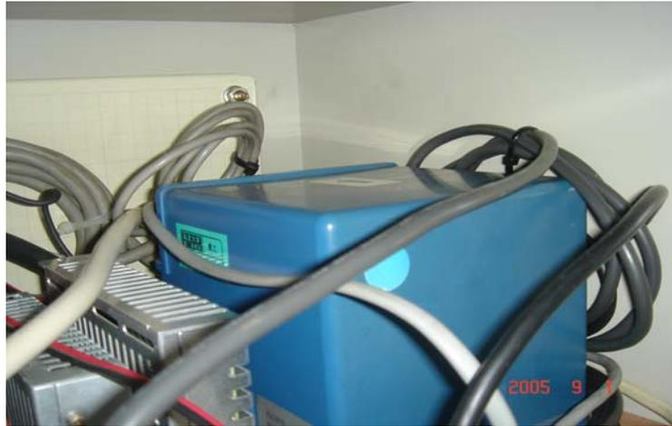
Fig. 5.4 Fiber optic gyroscope used in the autonomous tractor
