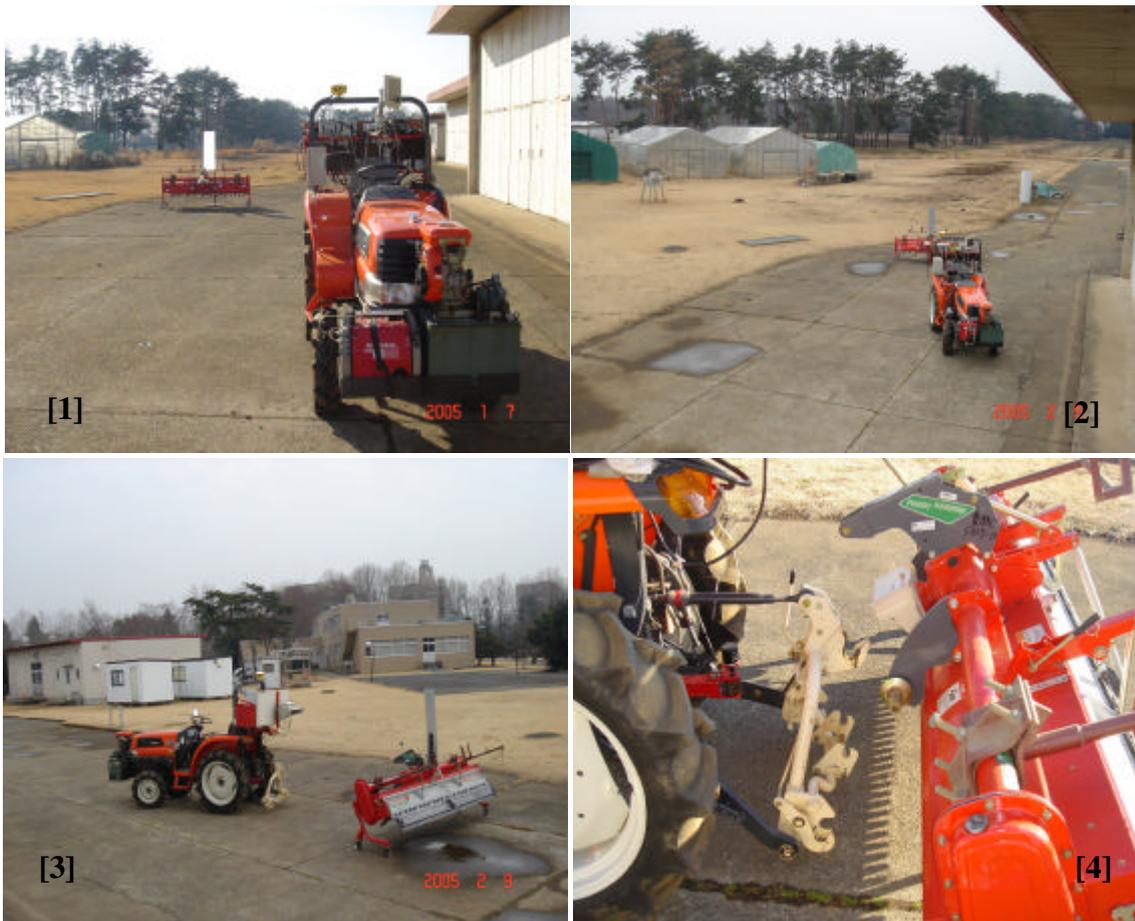
Fig. 7.4 Stages of approach toward the implement using experimental autonomous tractor
