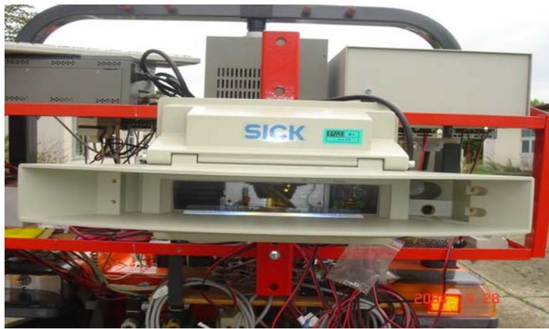
Fig. 5.6 The SICK LMS 211 laser range finder used in the autonomous tractor
