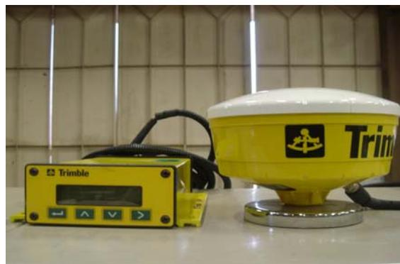
Fig. 5.7 Single receiver differential GPS used in the autonomous system
