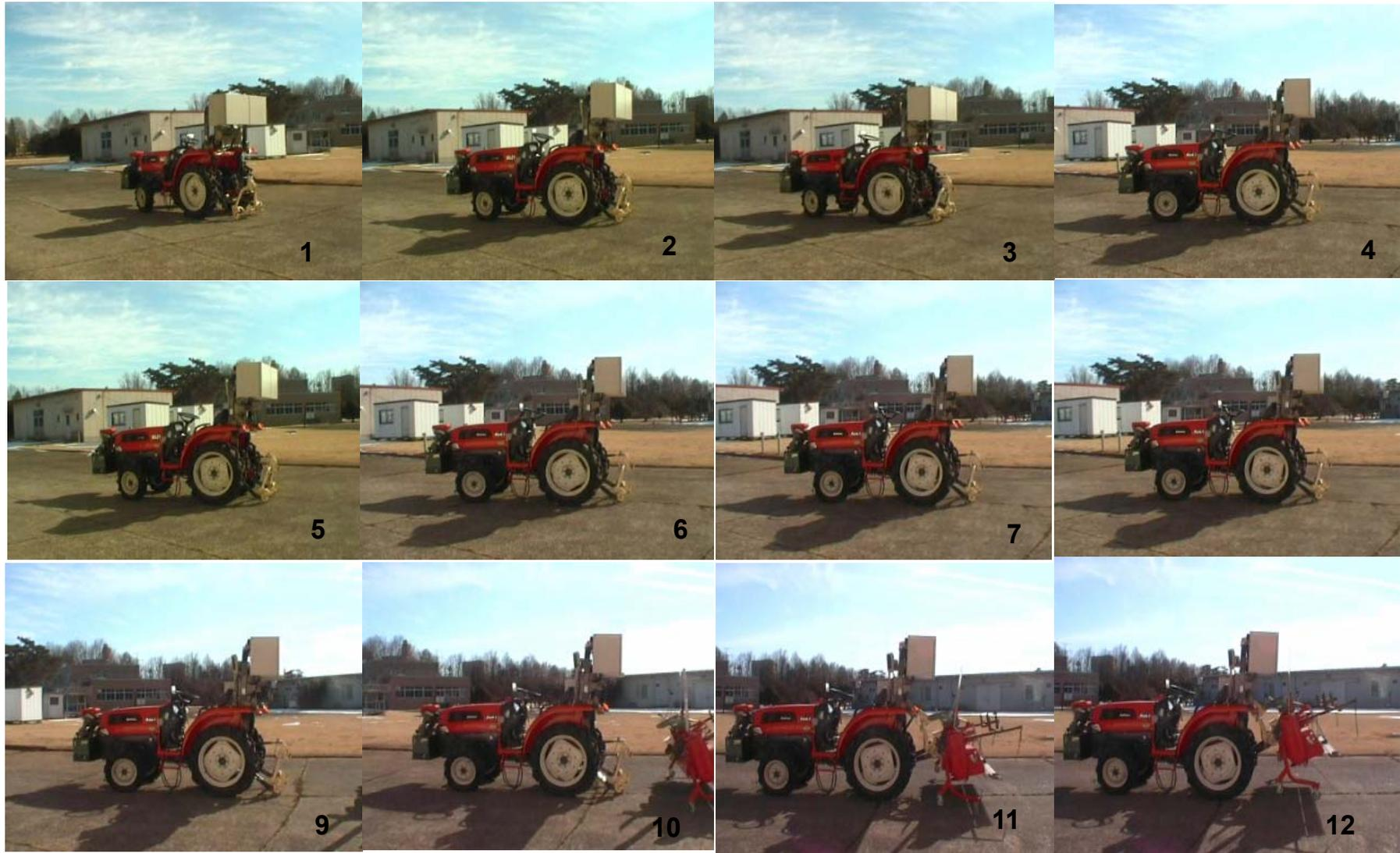
Fig. 9.9 Stages of automatic coupling with the implement using two reflectors (Implement at left)
