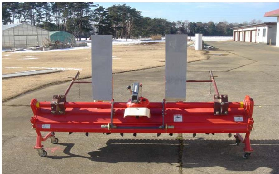
Fig. 9.5 Placement of two reflectors on the paddy harrow
