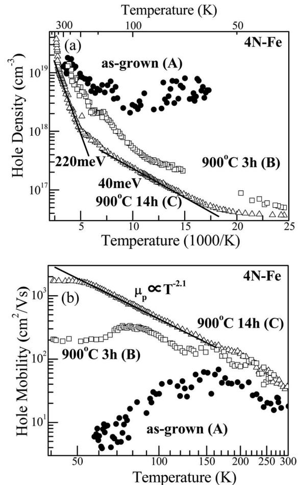
FIG. 2. Temperature dependence of (a) hole density and (b) hole mobility of the  $\beta$ -FeSi<sub>2</sub> films formed with 4N-Fe prepared using different annealing conditions.
