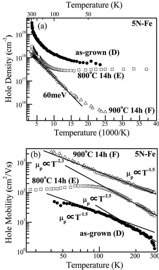
FIG. 3. Temperature dependence of (a) hole density and (b) hole mobility of the  $\beta$ -FeSi<sub>2</sub> films formed with 5N-Fe prepared using different annealing conditions.
