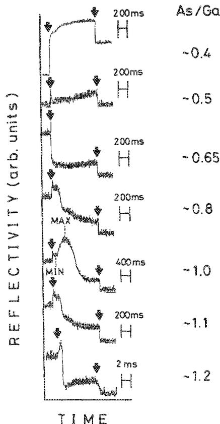
FIG. 1. TROR signals for various amorphous GaAs on Si samples with As/Ga ratios from 0.4 to 1.2 during laser irradiation. Laser power is 5.8 W and the temperature is estimated to be  $\sim 380^\circ\text{C}$ .
