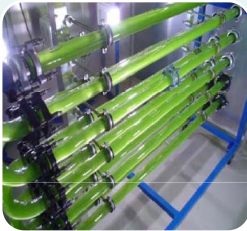
Tubular photobioreactor High efficiency but high cost
