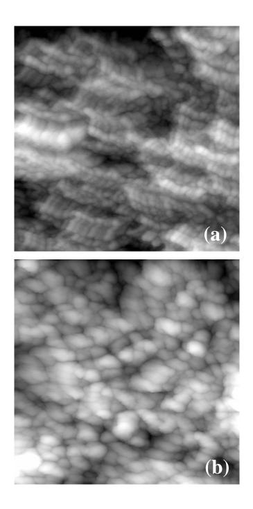
Fig. 7. STM surface images for (a) a Cu/Ta film with  $t_{\rm Cu}$  = 10 nm and (b) a Ta/Cu/Ta film with  $t_{\rm Cu}$  =30 nm. The X-Y scale is 1000 nm and the height scale is about 50 nm for the both images.
