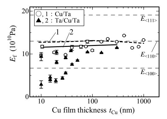
Fig. 4. The  $E_{\rm f}$  vs.  $t_{\rm Cu}$  data observed for as deposited Cu/Ta films and Ta/Cu/Ta films. The dashed curve 1 and the solid curve 2 are the theoretical values of  $E_{\rm f}$  estimated by taking into account the crystallographic texture (Fig. 3(a)) and the internal stress (Fig. 3(c)).  $E_{< hkl>}$  indicates the Young's modulus of Cu along the < hkl> direction.
