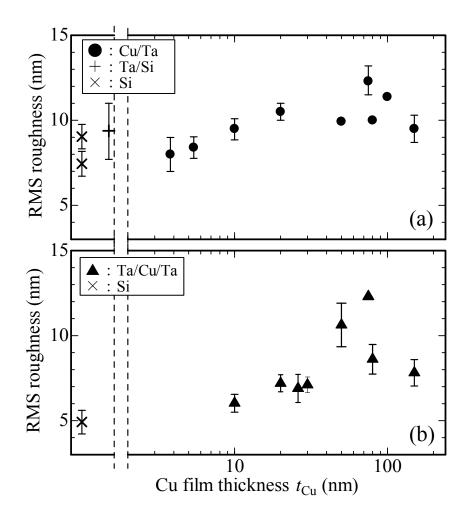
Fig. 8. The Cu film thickness dependence of the root-mean-square (RMS) roughness estimated from the STM surface images for (a) Cu/Ta films and (b) Ta/Cu/Ta films. The data observed for a Si reed substrate after etching and a Si reed substrate with a 30 nm Ta buffer layer are also shown.
