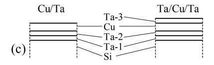
Fig. 1 Schematic diagrams: (a) a Si substrate, (b) a measurement setup, (c) cross sectional views of Cu/Ta and Ta/Cu/Ta films.
