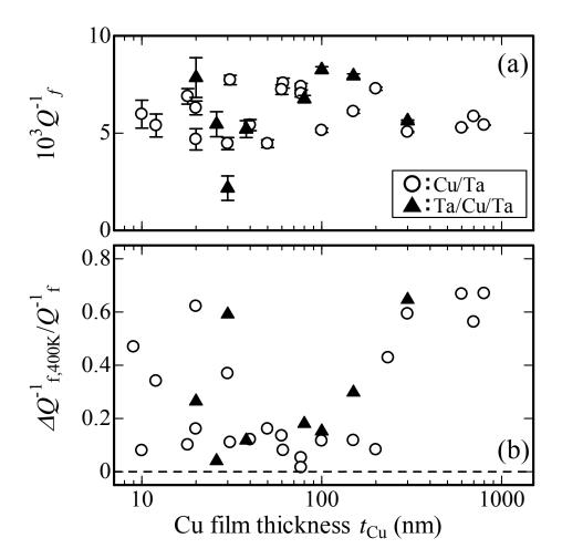
Fig. 6. (a) The  $Q^{-1}_f vs. t_{\text{Cu}}$  data and (b) the  $\Delta Q^{-1}_{f,400\text{K}} vs. t_{\text{Cu}}$  data observed at 300 K for Cu/Ta films and Ta/Cu/Ta films. See text for details.
