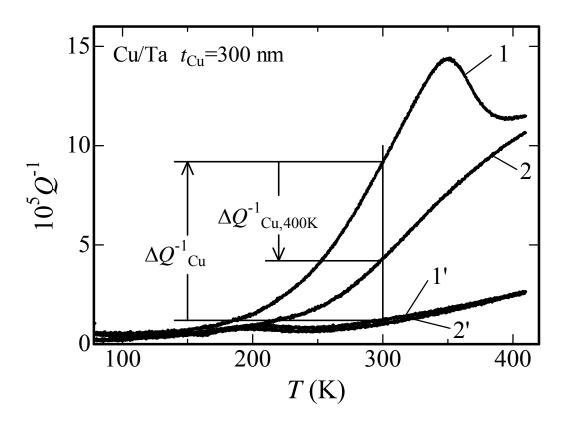
Fig. 5. Examples of the  $Q^{-1}$  vs. T data observed for a Si-reed with a 30 nm thick Ta buffer layer alone in the as deposited state (1') and after warm up to ~400 K (2') and those observed for a Si-reed with a 30 nm thick Ta buffer layer and 300 nm Cu specimen film in the as deposited state (1) and after warm up to ~400 K (2).
