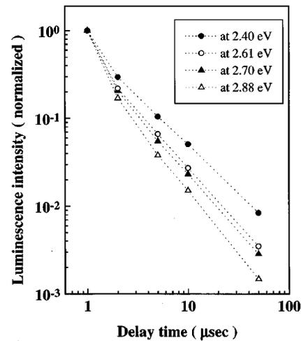
FIG. 7. Decay behaviors at various photon energies in the luminescence band of ZnS:(Ag, Al) nanoparticles. These data were obtained from Fig. 5.
