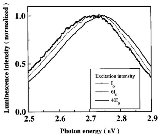
FIG. 9. Luminescence spectra of ZnS:(Ag, Al) nanoparticles for various excitation intensities at 10 K. The excitation was done by the 325.0 nm line (photon energy 3.81 eV) of a He–Cd laser.  $I_0$  is the lowest excitation intensity.
