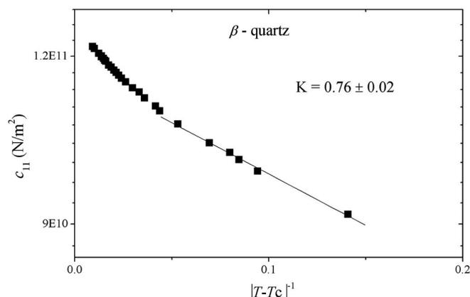
FIG. 5. The plot of  $c_{11}$  against  $|T-T_c|^{-1}$ . The value of  $K=0.76\pm 0.02$  is obtained from the slope.
