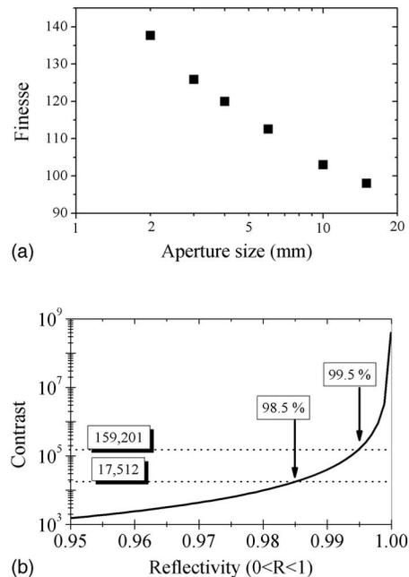
FIG. 2. (a) Aperture size dependence of obtained finesse. (b) A calculated curve of contrast as a function of reflectivity.
