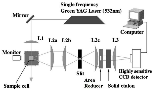
FIG. 1. Schematic diagram of the experimental setup. The mechanically stable solid etalon has been combined with the highly sensitive CCD detector. The AR has been set in front of the etalon for selecting the high flatness area of the etalon and lowering the kinetic broadening effect.
