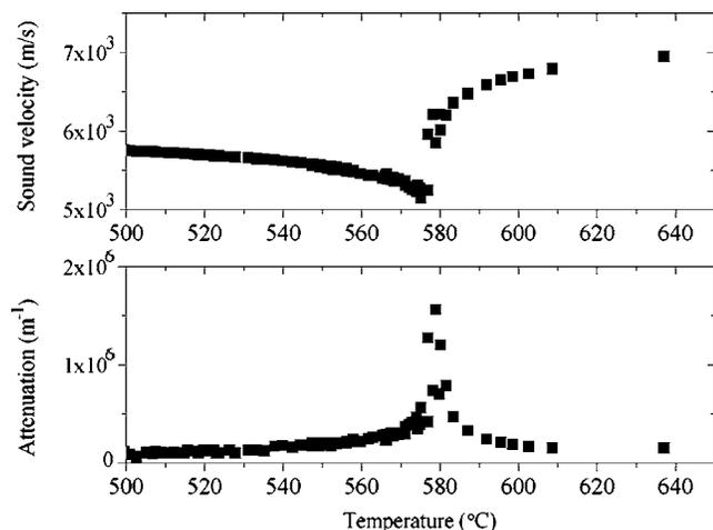
FIG. 4. Temperature dependences of sound velocity and attenuation of LA in a quartz crystal along the [010] axis.
