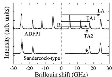
FIG. 3. Brillouin spectra of a quartz crystal at room temperature using the ADFPI with FSR of 30 GHz and using the Sandercock-type spectrometer.  $R$  denotes the elastic scattering (Rayleigh) component. The abbreviations of LA, TA1, and TA2 denote the Brillouin components scattered by the longitudinal acoustic phonon and two transverse acoustic phonon, respectively.
