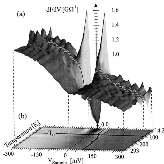
FIG. 3. (a) Three dimensional view of the conductance data shown in Fig. 2. The highlighted curve is the spectrum measured at  $T_c$ . (b) Projection onto the energy-temperature plane. The line at positive bias indicates the position of the positive bias conductance peak which clearly shifts to higher energies above  $T_c$ .
