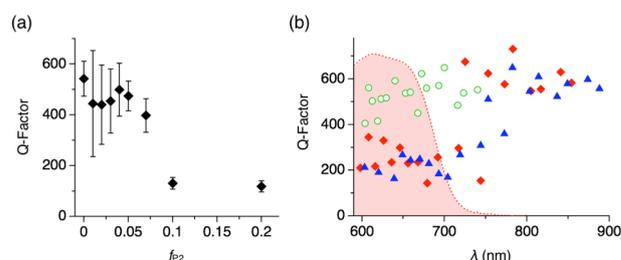
**Fig. 4.** (a) Plot of the average Q-factor versus  $f_{P2}$ . (b) Plots of Q-factors of each WGM PL line for microspheres with  $f_{P2} = 0$  (circle), 0.01 (square), and 0.02 (triangle). The red-colored area indicates photoabsorption spectrum of a  $\text{CHCl}_3$  solution of **P2**.
