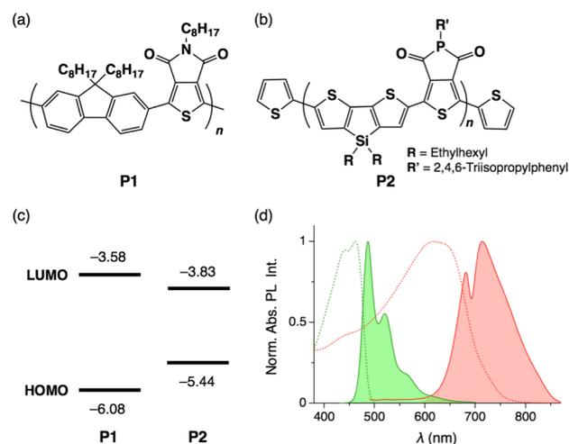
**Fig. 1.** Chemical structures of **P1** (a) and **P2** (b). (c) HOMO and LUMO energy levels of **P1** and **P2** with respect to the vacuum level. (d) Photoabsorption (broken lines) and PL (solid lines) spectra of **P1** (green) and **P2** (red) in CHCl<sub>3</sub>.
