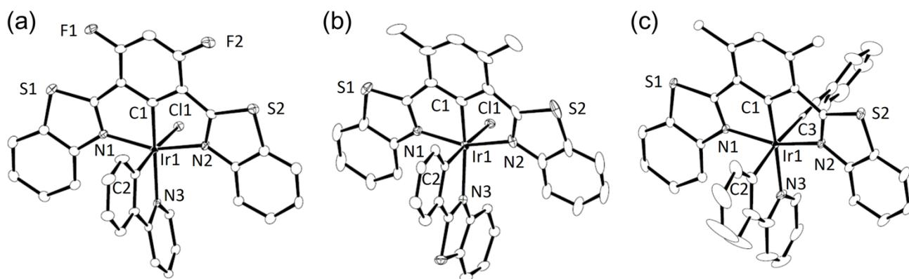
**Fig. 2.** Crystal structures of (a) **2**, (b) **3**, and (c) **4**. Hydrogen atoms and solvating molecules are omitted for clarity. The thermal ellipsoids are at the 30% levels.
