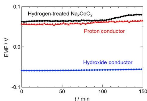
**Figure 4.** EMF measured by the water vapor concentration cell using the hydrogen-treated  $\text{Na}_x\text{CoO}_2$  disk, a proton-exchange membrane (Nafion NRE-212), or a hydroxide-exchange membrane (Tokuyama A201) as the electrolyte.
