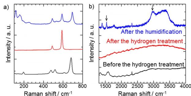
**Figure 2.** Raman spectra of  $\text{Na}_x\text{CoO}_2$  before and after the hydrogen treatment, and after its treatment followed by humidification. Spectra at lower and higher wave numbers are shown in (a) and (b), respectively.
