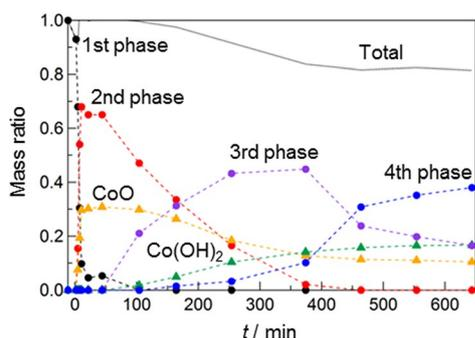
**Figure 1.** Time evolution of the mass ratios of crystal phases, which have been obtained by the Rietveld analysis of SXPd data under chemical reactions in  $\text{Na}_x\text{CoO}_2$ . The ratio of the first phase before the hydrogen treatment is set at 1.0.
