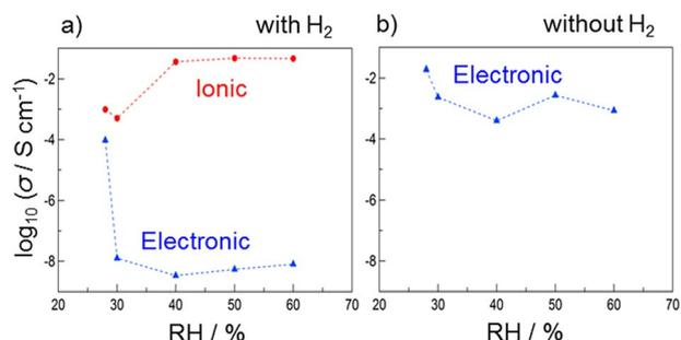
**Figure 3.** Ionic and electronic conductivities  $\sigma$  at 25 °C as a function of relative humidity (RH) on (a) the hydrogen-treated and (b) untreated  $\text{Na}_x\text{CoO}_2$  disks. No significant ionic conductivity is observed in the untreated disk.
