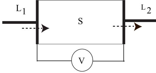
FIG. 1: Schematic set-up of the Kamerlingh Onnes's experiment. A specimen of mercury,  $S$ , is connected to leads,  $L_1$  and  $L_2$ , and the voltage drop is measured by feeding a current through the leads.
