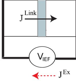
FIG. 4: Schematic set-up we consider for the Hamiltonian in Eq. (16).  $V_{\text{IEF}}$  denotes the voltage produced by the impressed electromotive force. A dc supercurrent flows through each superconductor in the junction as in the specimen in the Onnes's experiment depicted in Fig. 1.
