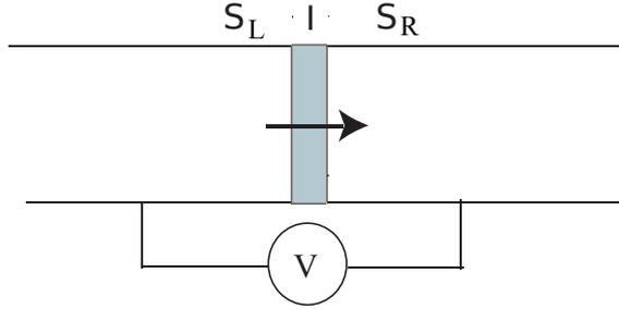
FIG. 2: Schematic set-up of the Josephson junction for which Josephson assumed in the predictions. 'S<sub>L</sub>' and 'S<sub>R</sub>' indicate the superconductor parts of the junction. The weak link is denoted as 'I'.
