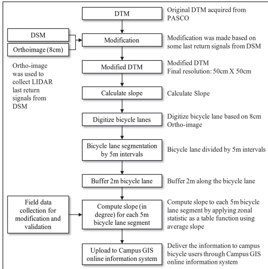
Fig. 3 Overview of data processing steps and methodology
