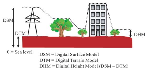
Fig. 1 Illustration of DSM, DTM and DHM in LIDAR data processing
