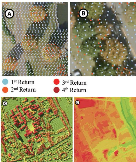
Fig. 4 Manual collection of ground hitting points from DSM to modify original DTM (A & B: 2nd, 3rd and 4th returns are more prominent in edge of the trees whose signals are returning from the ground, C: Shaded DSM, and D: Shaded DTM)
