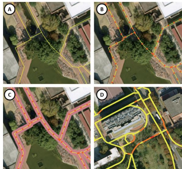
Fig. 5 Identification of bicycle lane slope process (A: Bicycle lane onscreen digitizing, B: Bicycle lane segmentation by 5m intervals, C: Buffer 2m each side of the bicycle lanes, and D: Calculate slope for each 2m buffered polygon by using zonal statistic as a table function in ArcGIS)
