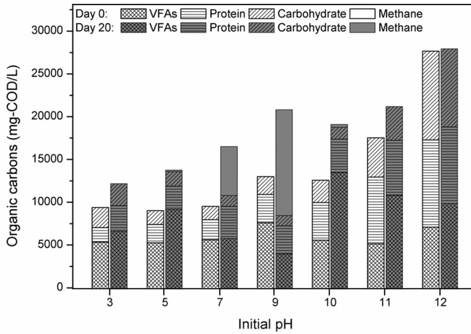
Figure 4 Composition of main organic carbons (soluble VFAs, protein, carbohydrate and accumulative methane) under different initial pH conditions on day 0 and day 20.
