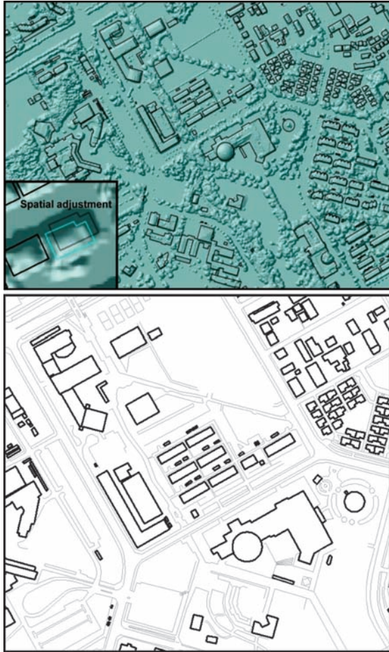
Fig. 3 Spatial adjustment performing between 2m above shaded Digital Height Model and building footprints
