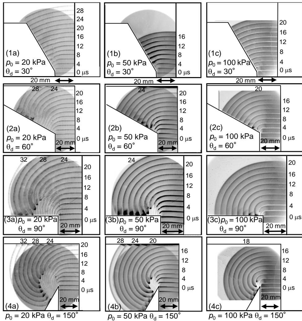
Fig. 4. Superimposed images of detonation diffraction in vertex
