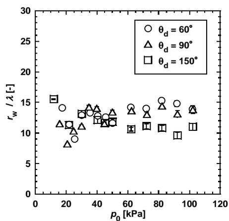
Fig. 6. Dependency of dimensionless wall reflection point on initial pressure
