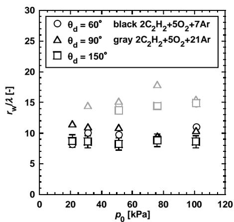
Fig. 7. Dependency of dimensionless wall reflection point on initial pressure ( $2C_2H_2+5O_2+7Ar$  &  $2C_2H_2+5O_2+21Ar$ )
