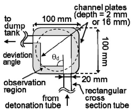
Fig. 1. Side view of the observation chamber and the observation region
