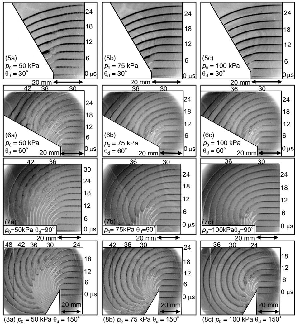
Fig. 5. Superimposed images of detonation diffraction in vertex
