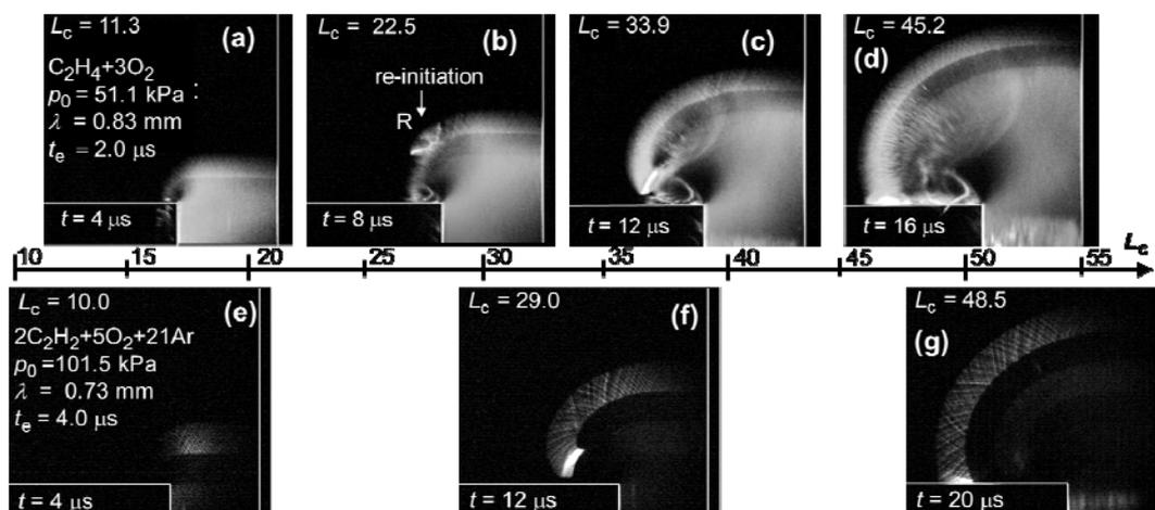
Fig. 2. MSOP image of detonation diffraction
