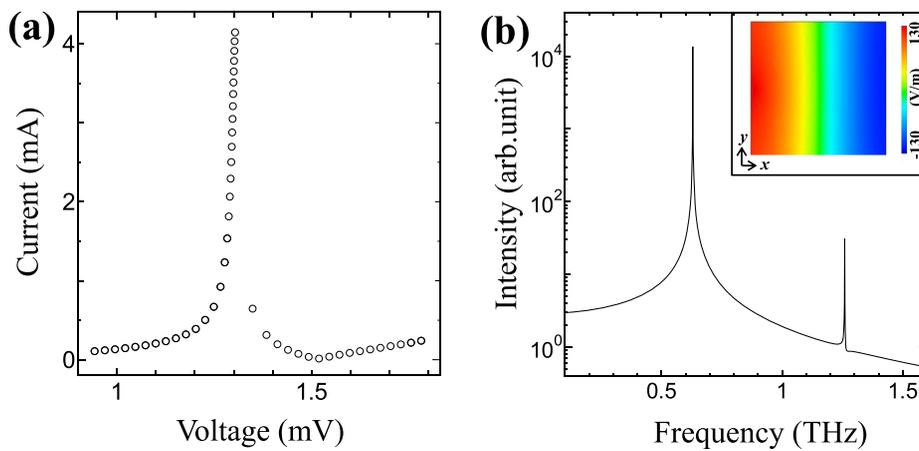
FIG. 3. (a) The displacement current as a function of voltage. (b) The frequency spectrum of the EM wave emitted by the antenna at 1.31 mV. An inset shows a snapshot of the oscillating part of  $E_z$  at 1.31 mV.
