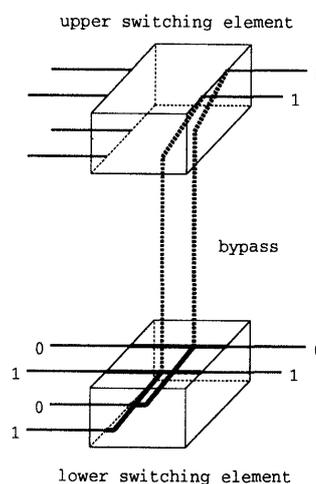
**Fig. 1**  $4 \times 2$  re-arrangeable upper switch and lower output switch with two bypasses.
