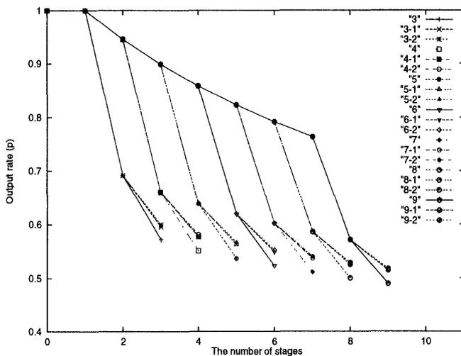
Fig. 3 Comparison of output rate for various hybrid dilated banyan networks depending on whether bypasses are used or not.
