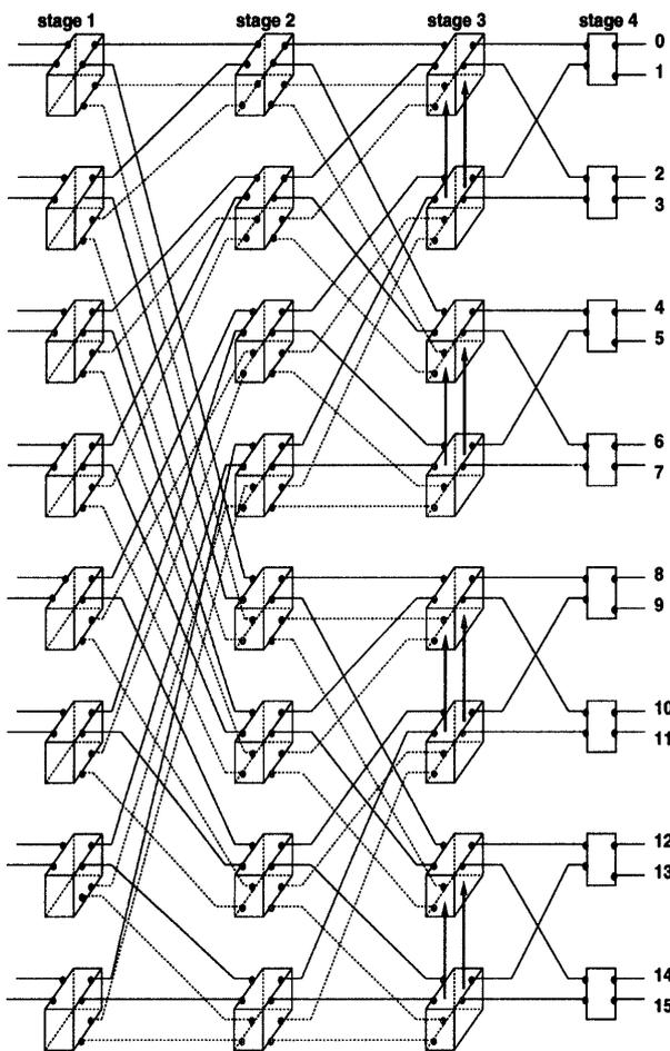
**Fig. 2** 16 × 16 hybrid dilated banyan network including two bypasses at the stage of 4 × 2 re-arrangeable switch.
