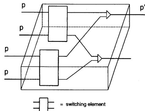
Fig. A.4 A 4 × 2 rearrangeable output switching element.
