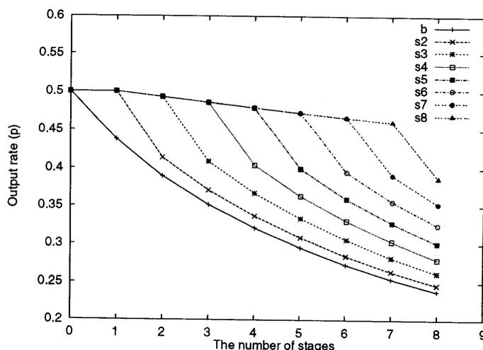
Fig. 9 Output rate vs. the number of stages at input rate = 0.50.
