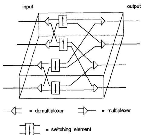
Fig. 3 A switching element for 2-dilated banyan network.
