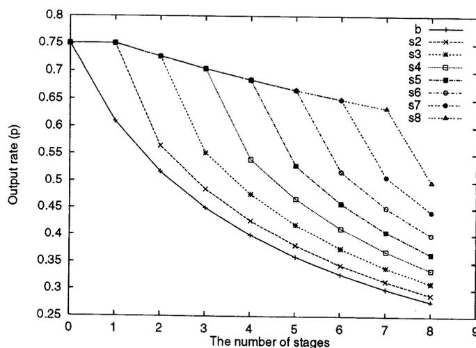
Fig. 8 Output rate vs. the number of stages at input rate = 0.75.
