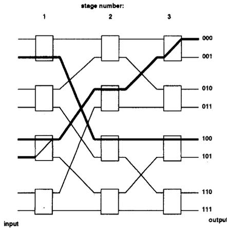
Fig. 2 8x8 banyan network with three stages.
