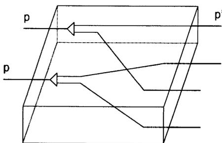
Fig. A.3 A 2 × 4 rearrangeable input switching element.
