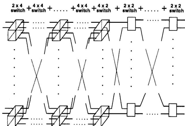
Fig. 5 The structure of hybrid dilated banyan network.
