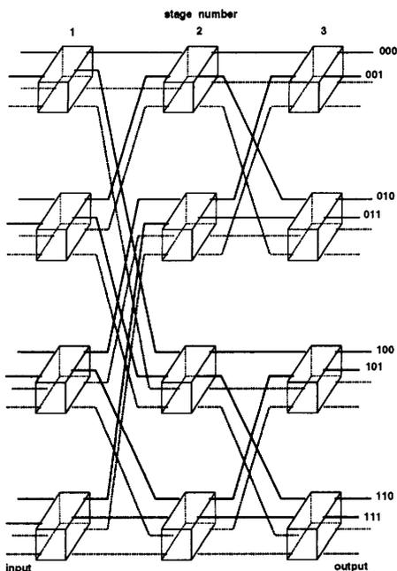
Fig. 4 2-dilated 8x8 banyan network with three stages.
