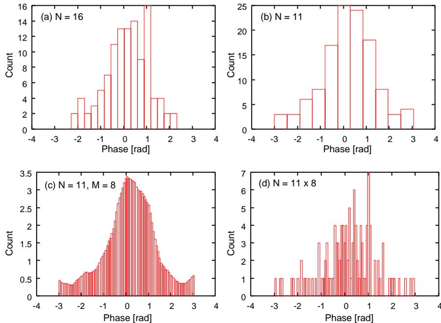
Fig. 3. Comparison of histograms with different number of histogram bins.  $N$ : number of histogram bins,  $M$ : the number of histograms used in the averaging process. The histogram bin width of each histogram is determined by (a) the phase noise and (b), (c) the Freedman & Diaconis rule. (c) is the averaged shifted histogram using eight histograms. (d) is a conventional histogram with a histogram bin width equivalent to that of the histogram in (c).
