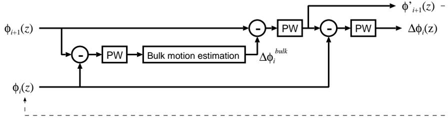
Fig. 2. The diagram of the bulk motion compensation algorithm.  $\phi_i(z)$ ,  $\phi'_i(z)$ : phases of  $i$ -th A-line before compensation and after compensation, respectively,  $\Delta\phi_i(z)$ : phase differences,  $\Delta\phi_i^{bulk}$ : the phase difference corresponding to the phase shift from 0-th A-line due to the bulk motion of the sample. PW: phase wrapping process.
