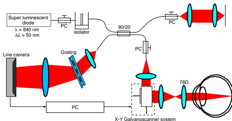
Fig. 1. Schematic of a high-speed spectral-domain OCT system
