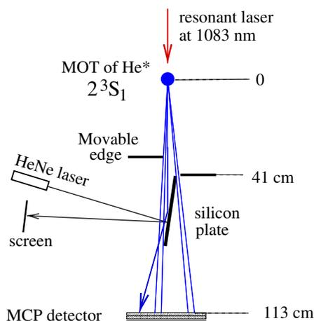
FIG. 2 (color online). Cross-sectional view of the experimental setup.
