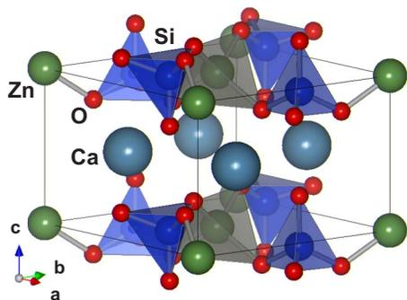
FIG. 1. (Color online) Crystal structure of  $\text{Ca}_2\text{ZnSi}_2\text{O}_7$ .
