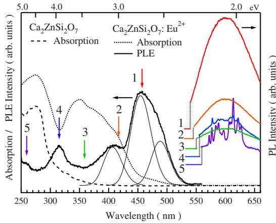
FIG. 3. (Color online) PLE and PL spectra of  $\text{Ca}_2\text{ZnSi}_2\text{O}_7:\text{Eu}^{2+}$  phosphor. The PL spectra were taken at the excitation wavelength between 260 and 460 nm. Emission was monitored at 600 nm for the PLE spectrum. Here, the lowest energy band in the PLE spectrum is decomposed into three Gaussian components. Dotted and dashed lines show the absorption spectrum for the phosphor and the pure matrix, respectively.
