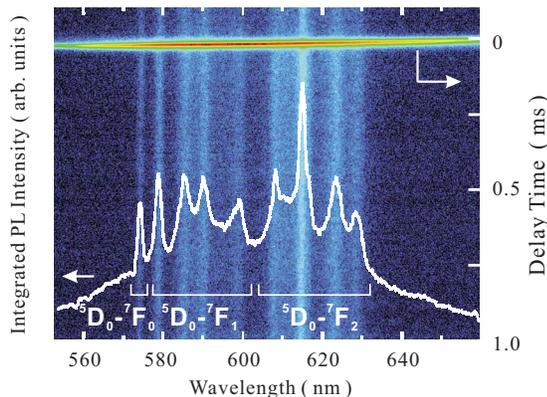
FIG. 5. (Color online) Integrated PL intensity spectrum and contour plot for a streak image with a delay time region of  $\leq 1$  ms. The excitation was performed by 266 nm femtosecond pulses at 298 K.
