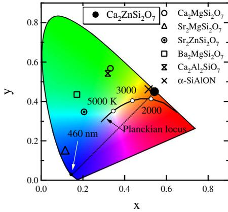
FIG. 4. (Color online) Chromatic coordinates for  $\text{Ca}_2\text{ZnSi}_2\text{O}_7:\text{Eu}^{2+}$  and several isomorphous compounds. The coordination for Ca- $\alpha$ -SiAlON is also plotted as a typical red-orange phosphor.
