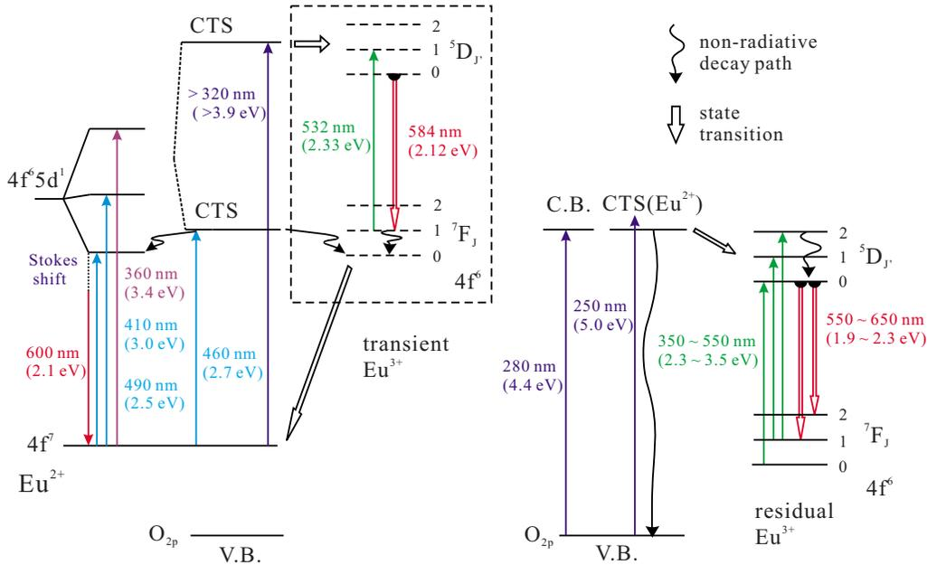
FIG. 11. (Color online) Energy diagram of  $\text{Ca}_2\text{ZnSi}_2\text{O}_7:\text{Eu}$ .
