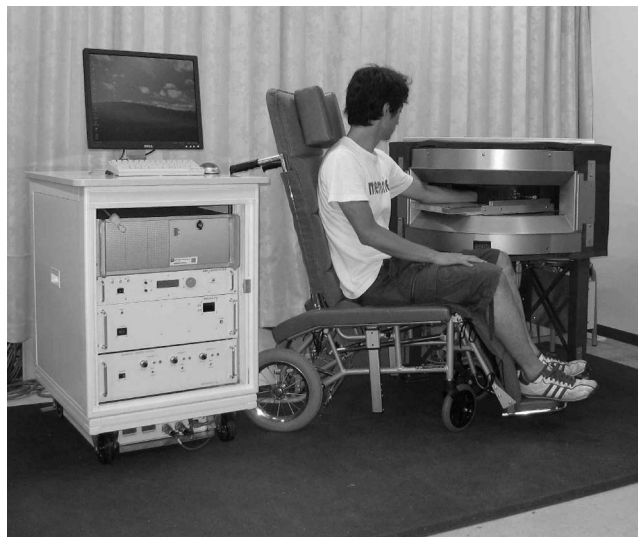
FIG. 1. Overview of the compact MRI system developed and installed in our laboratory.
