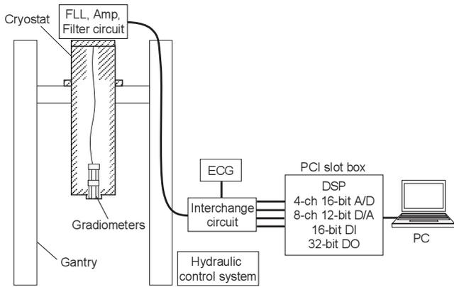
FIG. 2. Schematic diagram of the fMCG system.
