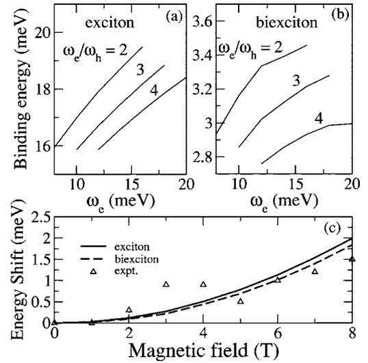
FIG. 4. Calculated binding energies of (a) exciton and (b) biexciton for various values of the confinement parameters  $\omega_e$  and  $\omega_h$  (see the text for details). The bottom panel (c) shows the magnetic field dependence of the exciton (solid line) and biexciton (dashed line) emission energies for  $\omega_e=12$  meV and  $\omega_h=4$  meV. The points (open triangles) denote experimental data for the exciton.
