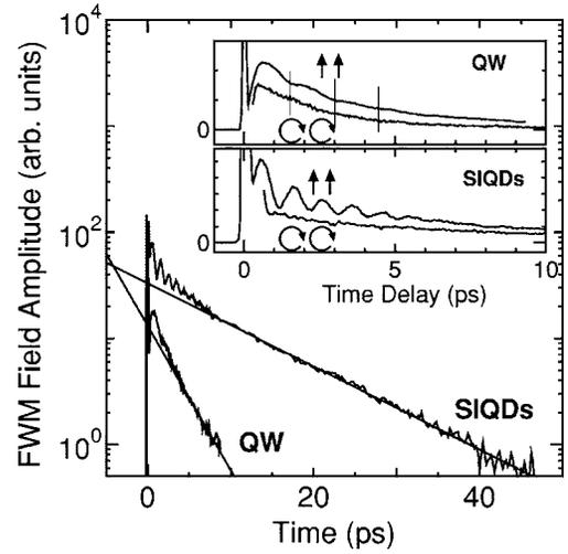
FIG. 2. The logarithmic plot of the FWM signal at the SIQDs peak and at the QW peak at 2 K. The decay time of the signal at SIQDs (QW) is 12 ps (3.2 ps). Inset: The polarization dependence of the FWM signal of the initial part.
