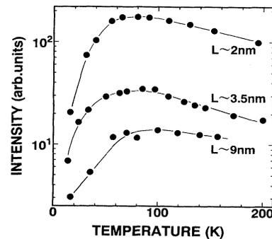
FIG. 6. Temperature dependence of the PL intensity in porous Si films of  $L \sim 2$ ,  $\sim 3.5$ , and  $\sim 9$  nm. The PL intensity increases with raising the temperature up to about 100 K and then decreases gradually.
