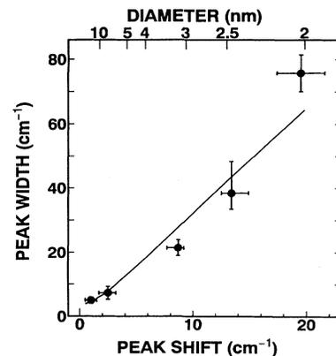
FIG. 3. The calculated relationship between the Raman width, the decrease of the Raman peak shift with respect to *c*-Si.  $L$  is the average diameter of Si crystallites.
