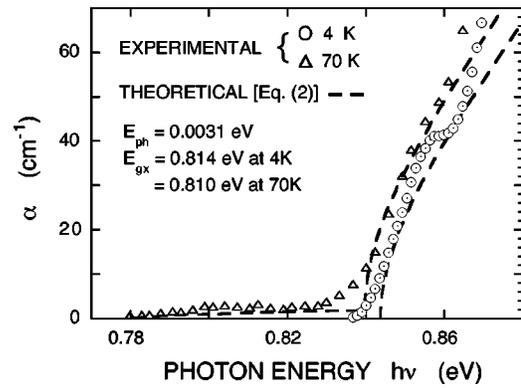
FIG. 3. The edge-absorption spectra of  $\beta$ -FeSi<sub>2</sub> at 4 and 70 K. The components associated with the phonon emission and absorption compared with the theoretical expression of Eq. (2), with the assumption of the one phonon energy of 0.031 eV.
