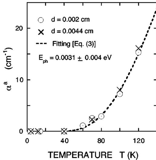
FIG. 2. Temperature dependence of the strength of absorption component  $\alpha^a$ . The phonon energy  $E_{ph}=0.031\pm 0.004$  eV was obtained from the fitting to Eq. (3).
