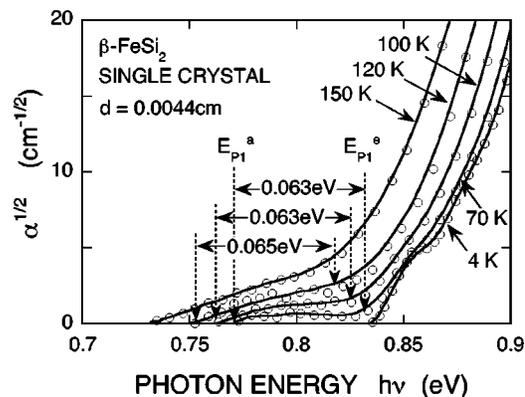
FIG. 1. The low-level absorption spectra near the absorption edge of single crystalline  $\beta$ -FeSi<sub>2</sub> at various temperatures.
